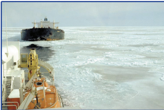
Photo 3.1: Escorting oil tanker through very close pack, heavily rafted grey ice.
