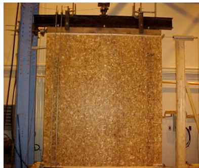
Determining strength of a proprietary stud wall
