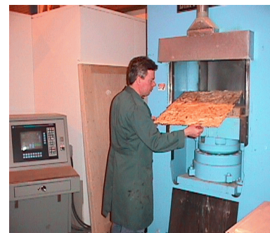
Wood composite panel research using state-of-the-art lab press
