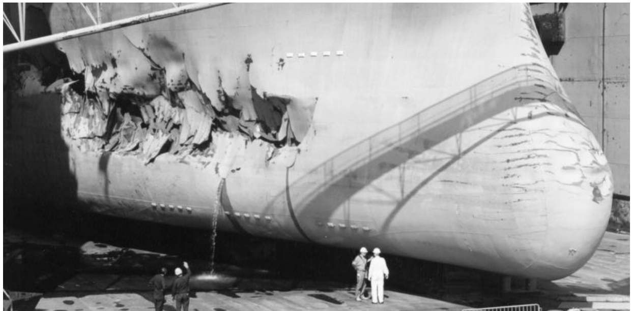
Figure 42 This Type D Bulk Carrier was damaged by ice in Hudson Strait
