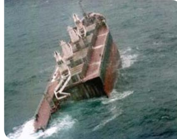
Substandard ship that cracked in half and sank
