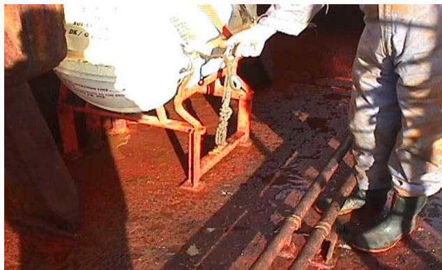
Seized liferaft release mechanism
