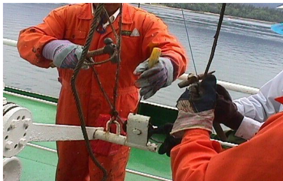
Lifeboat Launching device has to be pried open
