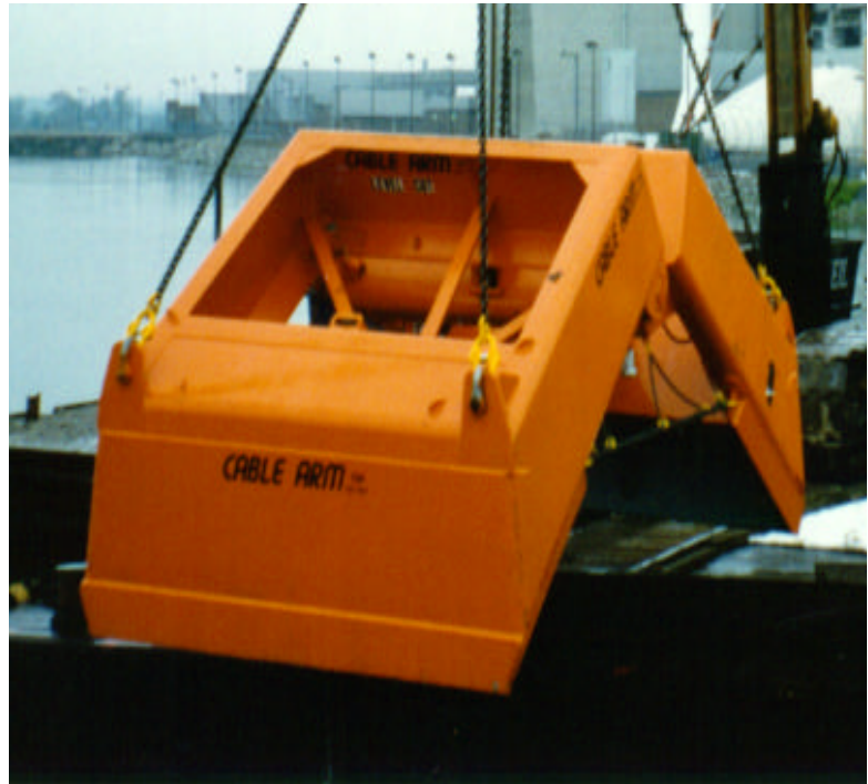
Cable Arm Environmental Clamshell used during the 1993 Pickering NGS project
