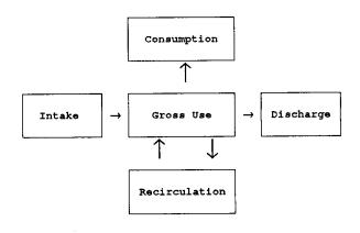
Figure 1. An industrial plant water system.
