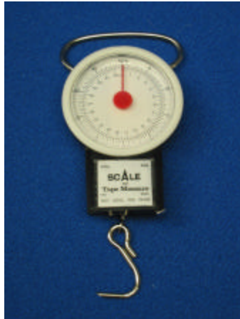
Figure 2. Spring-type fish scale used to measure seat belt slack.
