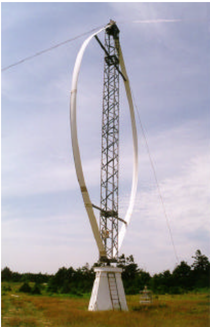
(caption 5 -The "dynamically soft" vertical axis turbine – "SoftVAWT")
