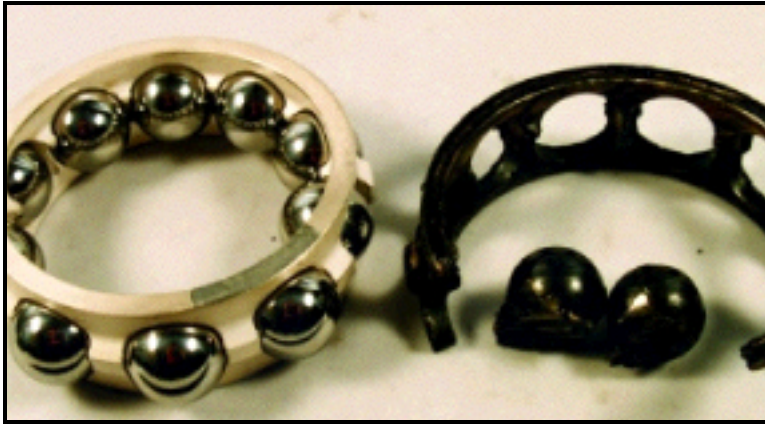
Comparison of a new bearing (left) with a bearing that has suffered from electrical discharge damage (right).
