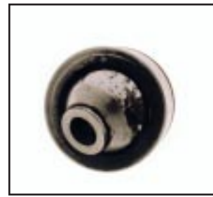
Right-hand rod end showing some pitting and wear on the ball.
