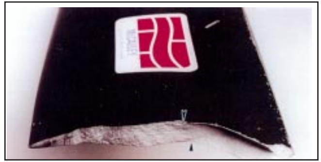
View of fracture surface showing the failure progression and start of the shearing (arrows).
