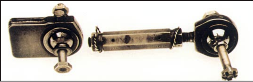
Failed tail rotor control rod assembly as received.
