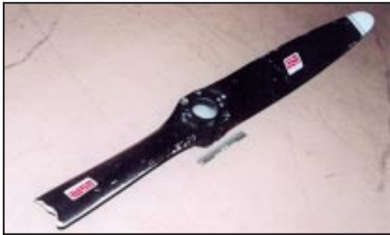
Propeller blade as received, missing the tip.
