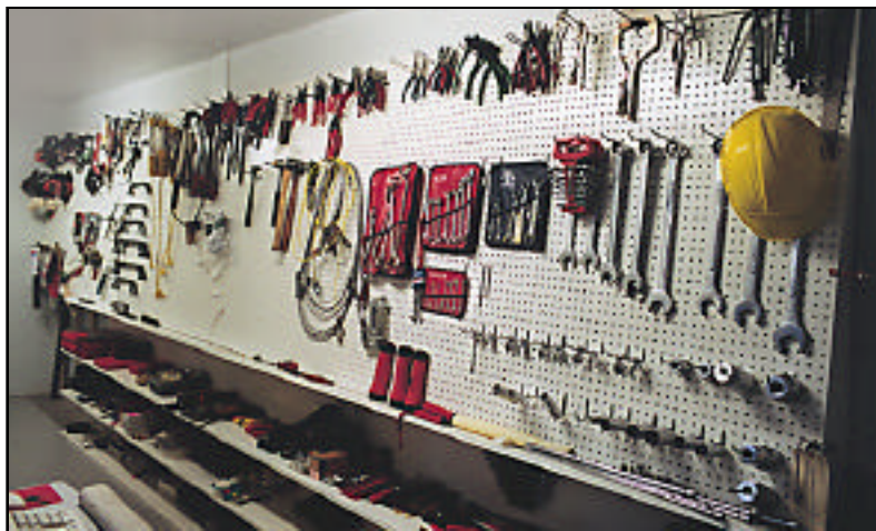
The quality of repairs often depends on locating the correct tool. The board above, inclined slightly out at the top, is an excellent way to locate and track tools where multiple users are involved. A silhouette or number system on the board can be used to quickly verify that no tools have been left in the work area after each day's use.
