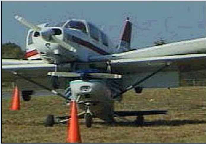
Classic demonstration of the visibility conflict between low- and high-wing light aircraft. Unbelievable midair collision at Plant City Municipal Airport, Florida, on December 11, 1999.
