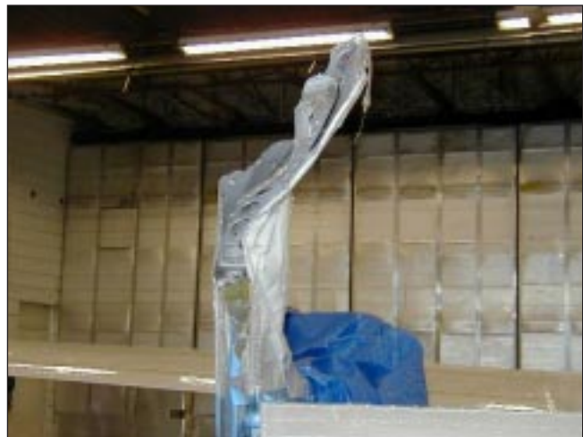
Close-up view of the Cessna 337 damaged left vertical stabilizer.
