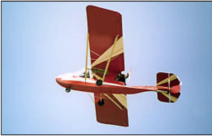
The Challenger ultralight shown above is similar to the Challengers involved in the accidents mentioned. This is a unique aircraft designed specifically for very slow flight operation and, as such, it has unique flying and control characteristics. For your safety, obtain dual training and experience prior to attempting solo flight in this aircraft type.
