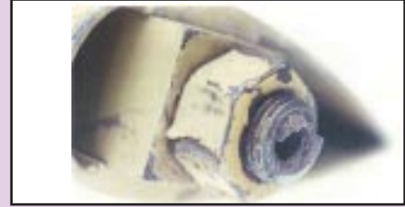
Close up of the fracture surfaces from the right strut of the accident aircraft.
