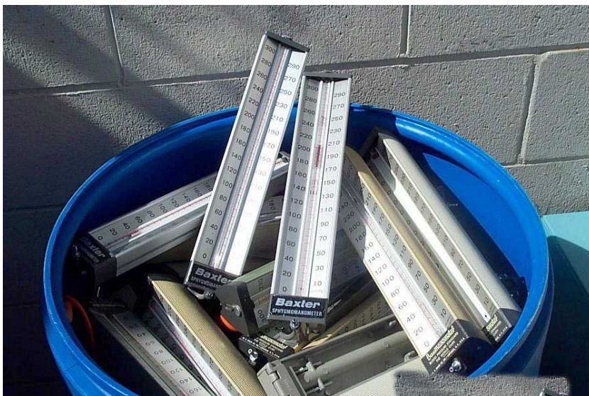
Figure 3 Unless recycled, the 90 sphygmomanometers, along with thermometers and bougies not seen, would have to be managed as hazardous waste at great expense. There are programs to exchange both bougies and sphygmomanometers. (Pollution Prevention Project Photograph)
