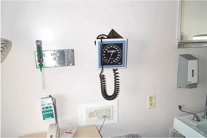
Figure 2 The bedside mercury sphygmomanometer has been replaced with an aneroid unit. (Pollution Prevention Project Photograph)
