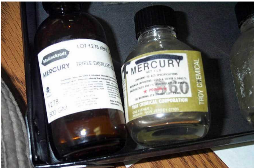
Figure 5 The bottle of "new" mercury (left) weighs 500 grams (454 grams is a pound). The waste mercury (right) was estimated at 0.3 pound. (Pollution Prevention Project Photograph)
