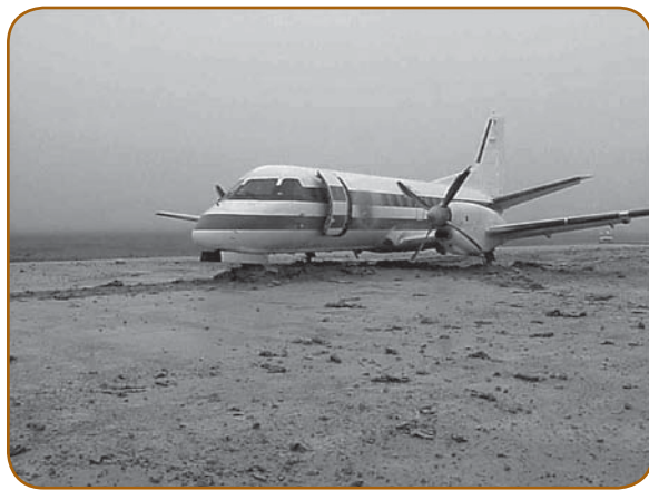
Example of an overrun that didn't become an accident due to a soft arrestor bed.
