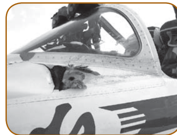
Birdstrike damage on a Snowbirds aircraft
