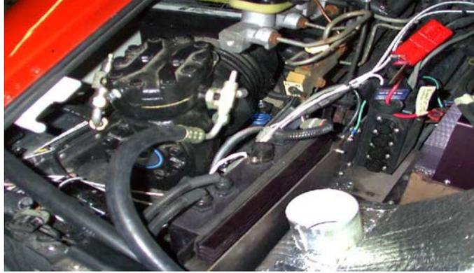
**Figure 1** *Installed compression unit*
