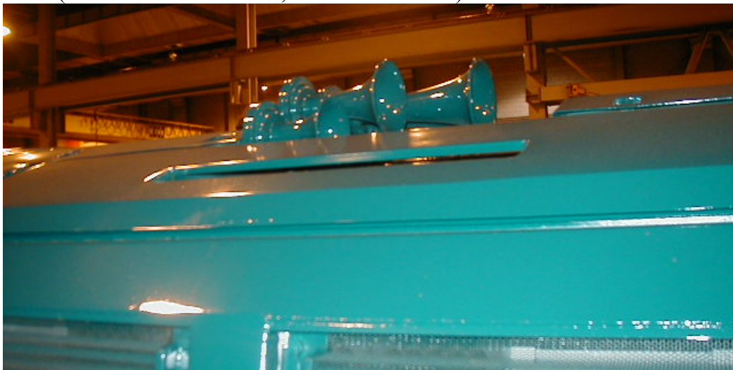
Locomotive Genesis – emplacement normal du klaxon
