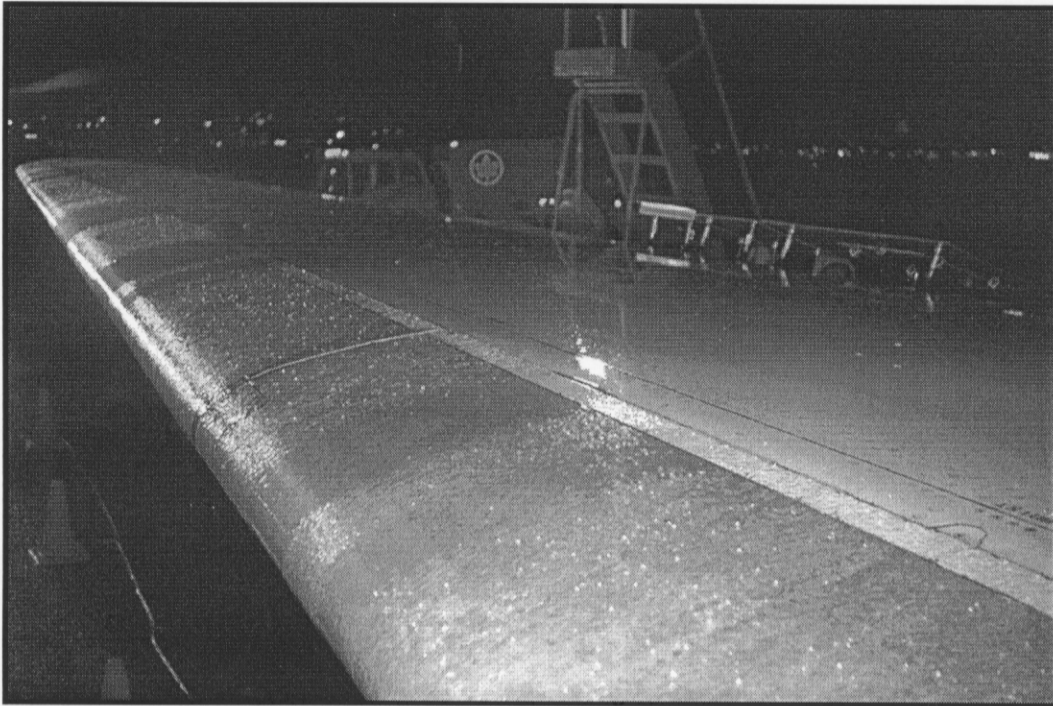
PHOTO 3.2 DC-9 WING SURFACE DURING FREEZING RAIN TESTS AT DORVAL (Feb. 28, '96) DURING FAILURE
