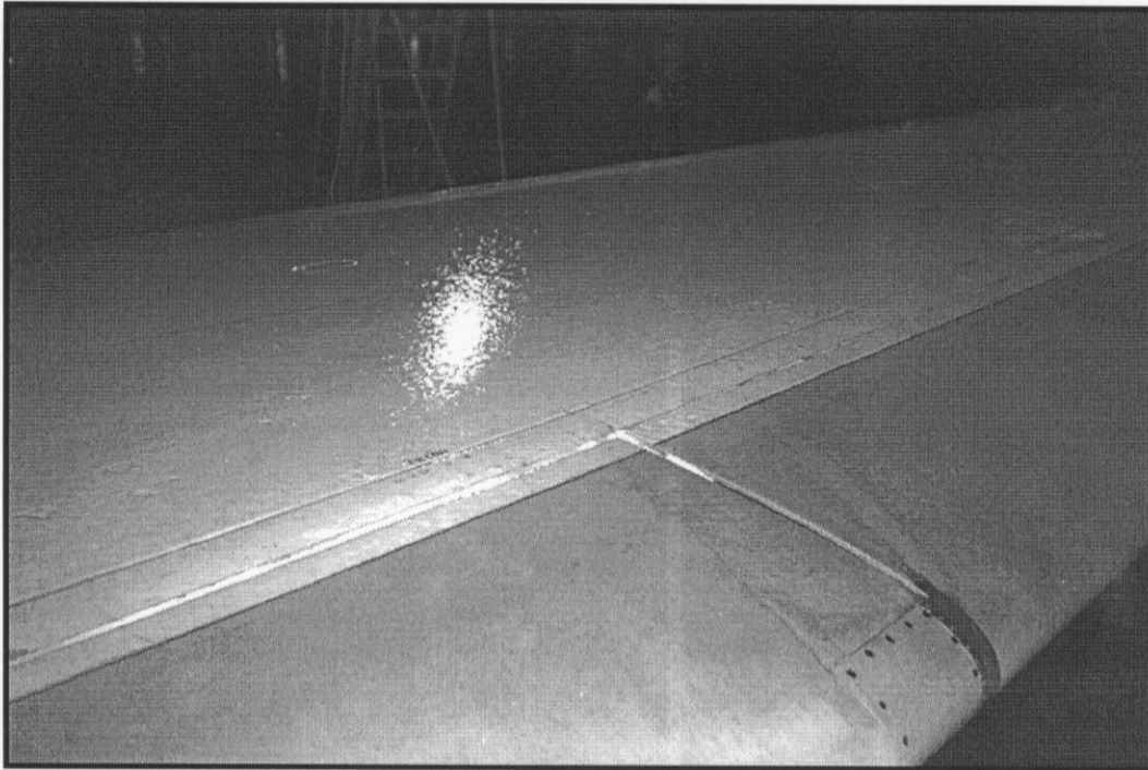
PHOTO 3.3 DC-9 WING SURFACE DURING FREEZING RAIN TESTS AT DORVAL (Feb. 28, '96) AFTER FAILURE
