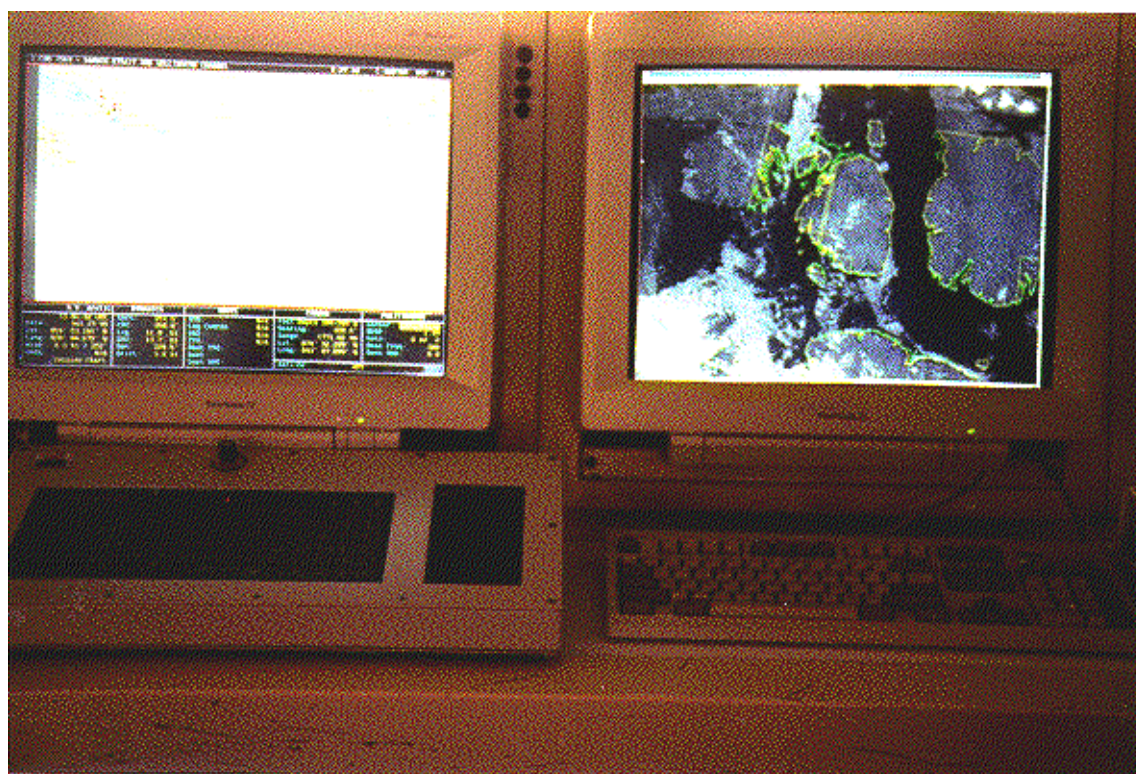
Figure 6-1 Bridge Installation of IceNav MRI System M.V. Arctic - October 1995
