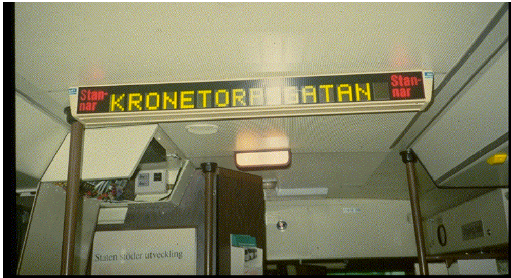
Figure 10 Displaying the name of the next stop inside a bus in Malmö, Sweden. The display is driven by the automatic vehicle location system (AVL) fitted to the bus. The red sign each side of the stop name is an indication that the next stop has been requested.
