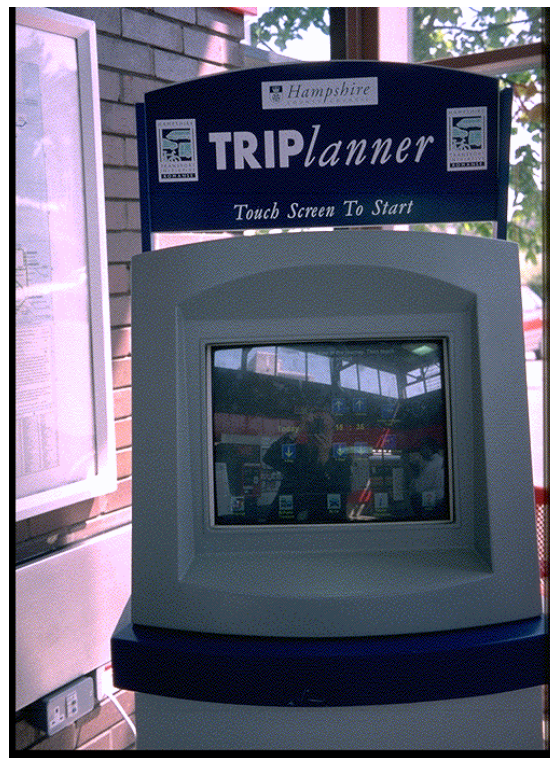
Figure 8 A trip planning information terminal. This example of a multi-modal trip planning terminal is at the main railway station in Southampton, England. It is operated through touch-screen controls and provides information on public transport services by bus, rail, air and ferry. For public transport or car journeys it gives details of the best route from a specified origin to destination. Once a route has been selected, detailed instructions can be printed for the traveller. The service is free to the public.
