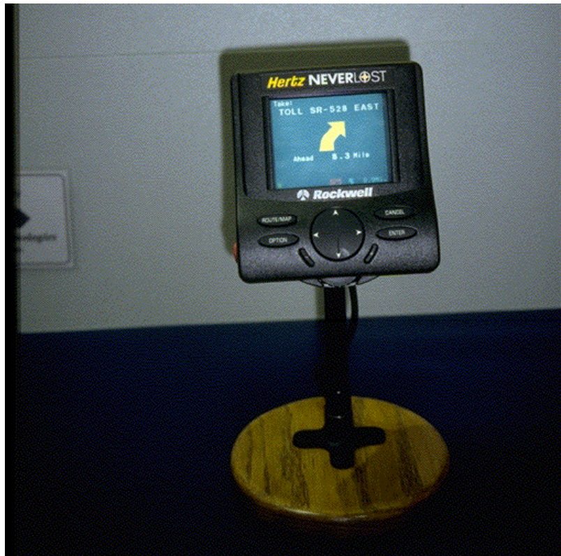
Figure 7 The Rockwell/Hertz "Neverlost" navigation system. This on-board navigation system provides either a map display or junction by junction directs from the present position of the vehicle to a selected destination. Audio instructions are given on the approach to each junction. This illustration shows an instruction to bear right onto the SR 528 East toll road in 0.3 miles.
