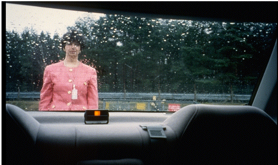
Figure 17 The Bosch ParkPilot obstacle warning system. The light array on the rear parcel shelf shows green, yellow, red or red flashing, depending on the distance to the nearest obstacle behind the car.
