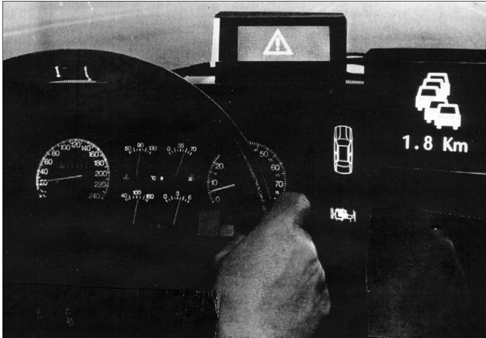
Figure 15 In-car signing in a driving simulator at Centro Recherche Fiat (Photo: Centro Recherche Fiat in ITS: intelligent transportation systems)
