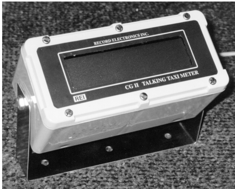
Figure 13 An easy-view “talking” taxi meter to assist visually and hearing impaired passengers
