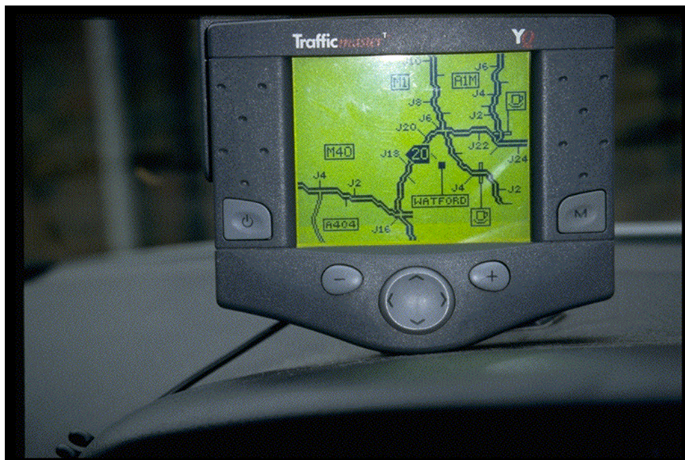
Figure 6 The Trafficmaster traffic information system in Britain. The system displays the speed of traffic on the motorway system, real time, at any points where the speed is less than 30 mph. This illustration shows the northwest quadrant of the M 25 London outer orbital motorway. The arrow with the number 20 in it indicates that at that point the traffic speed in the direction of the arrow has averaged 20 mph for the last three minutes. The display unit can be removed from the car; its battery provides about 8 hours of independent use as a hand-held unit.
