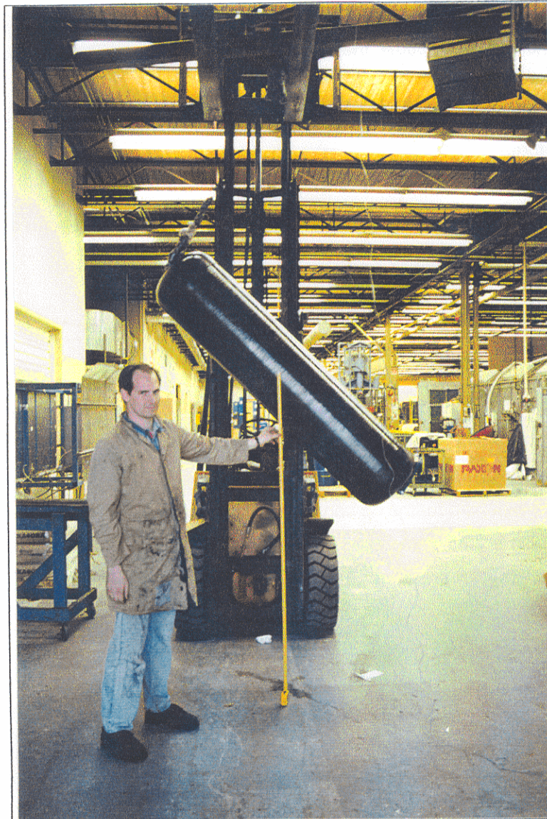
Figure 7.2: The 45° Drop Test
