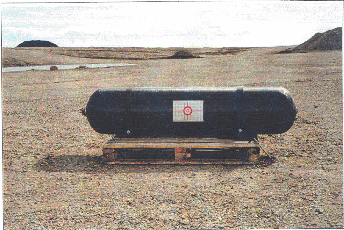
Figure 7.3: The Cylinder Set-up for the Penetration Test
