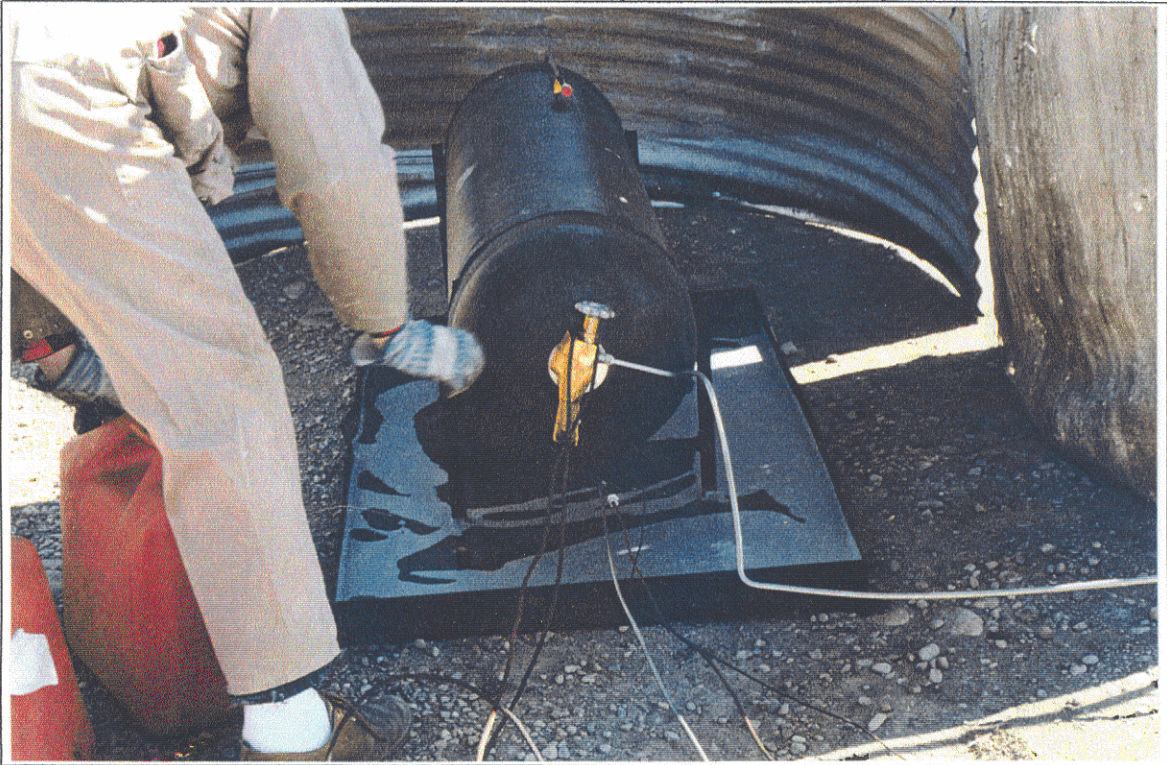
Figure 7.7: The Hydrogen Hybrid Cylinder Bonfire Set-up
