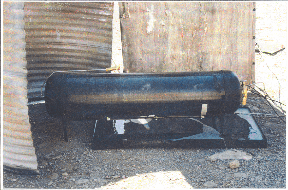
Figure 7.6: The Hydrogen Hybrid Cylinder Bonfire Set-up
