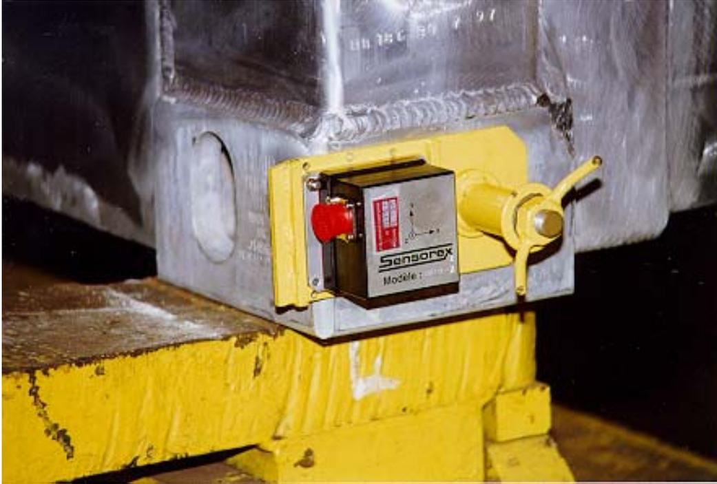
Figure 1. Accelerometer Mounting Location On Corner Casting
