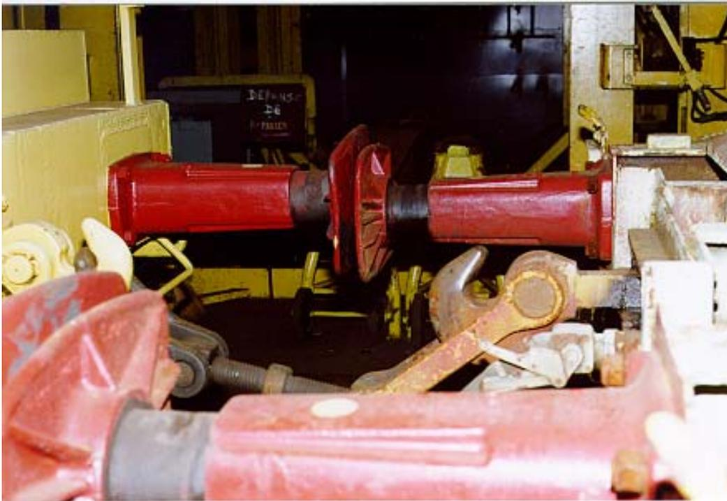
Figure 2. Buffers (Draft gear) and Couplers - European Style Equipment
