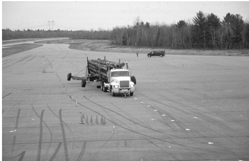
Figure 3. High speed lane change manoeuvre.
