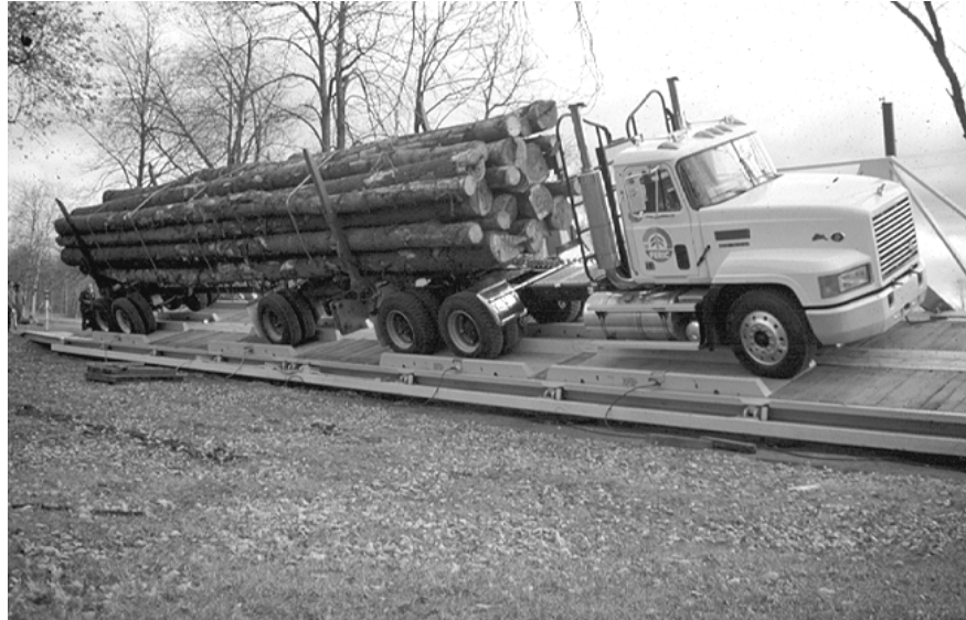
Figure 2. Tilt table testing of tandem tractor/jeep/tandem pole trailer.
