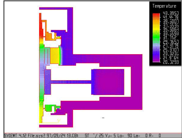
Figure 10 Modelled Steady State Thermal Map (ACES2 at 25,000 rpm)
