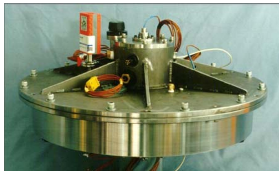
Figure 1 Attitude Control Energy Storage (ACES) System
