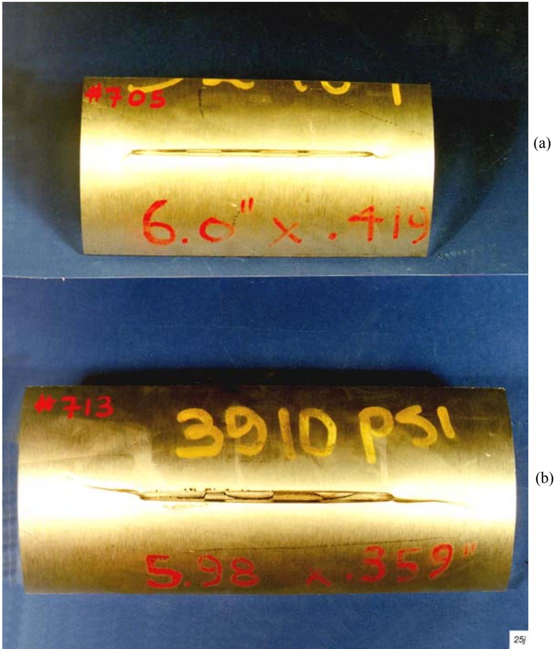
Figure A-11. Figures show the extension of the machined flaw along the length of the all-aluminum (AA6061-T6) Luxfer cylinders, observed during the hydraulic flawed cylinder burst tests:
