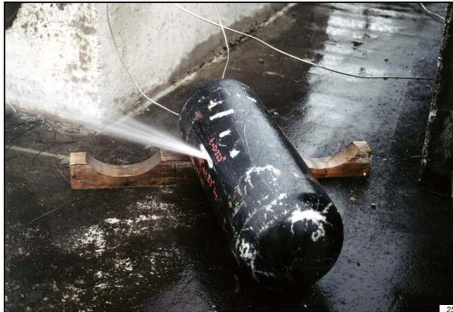
Figure A-9. An all-steel Faber cylinder with a 3.3" (84 mm) long axial flaw having a depth of approximately 80% of wall thickness leaked under a hydraulic pressure of 3,750 psi (25.85 MPa)
