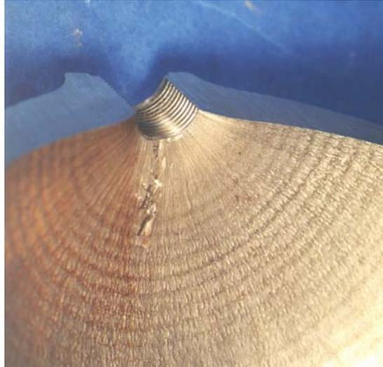
*Figure A-21. Photograph shows the location of an internal gouge mark (1.5 inch [38 mm] long and 0.2 inch [5 mm] deep) introduced at the neck area of an aluminum-lined hoop-wrap CNG Cylinder Co. cylinder by cold chiselling method prior to fatigue cycling.*
