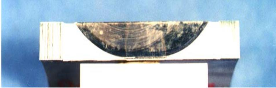
*Figure A-5. Photograph shows cross section of an axial external machined flaw introduced onto.*
