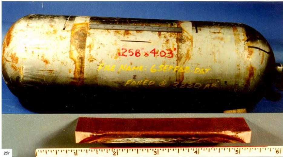
Figure A-4. Photograph shows location and cross section of machined flaw introduced onto the external surface of an all-steel Faber cylinder.
