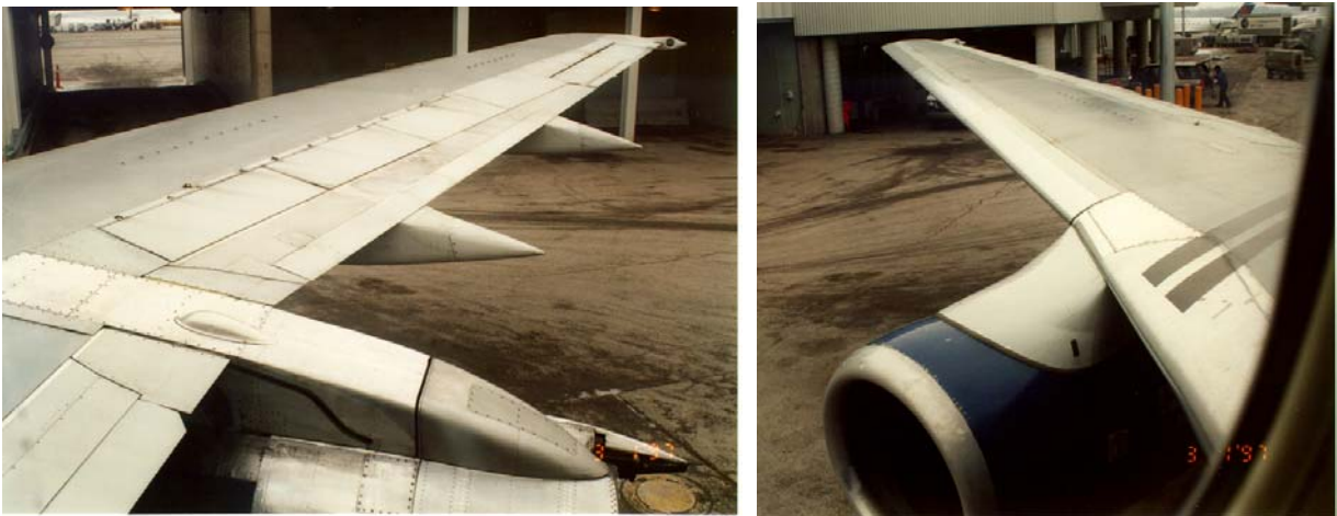
Figure 8.6 View of the Leading and Trailing Edge Sections of a Boeing 737 Wing From the Cabin
