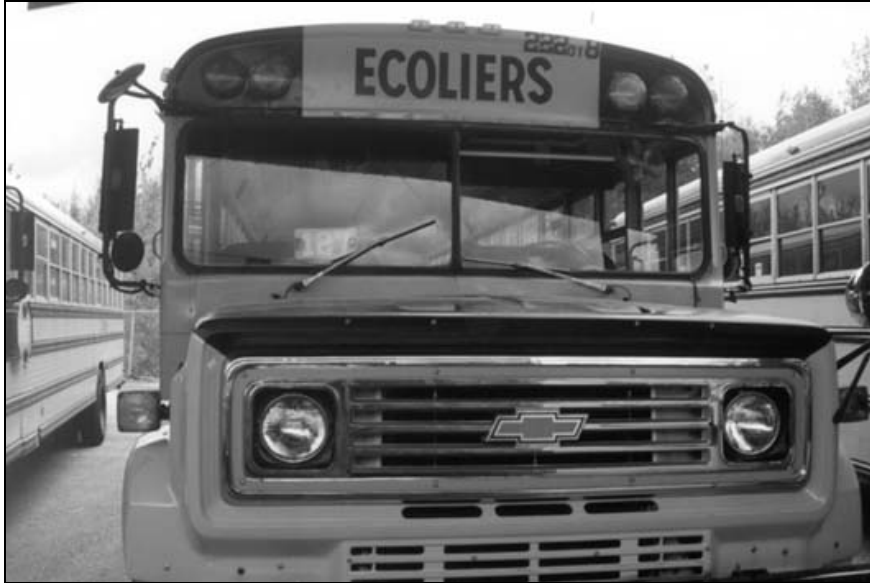
Figure 5 Long-nosed bus equipped with smaller sized hazard lights
