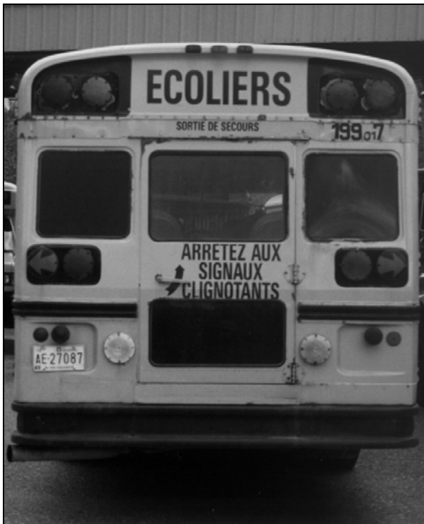
Figure 3 Eight-light system, rear view
