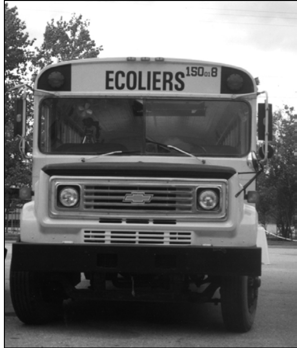
Figure 2 Four-light system, front view
