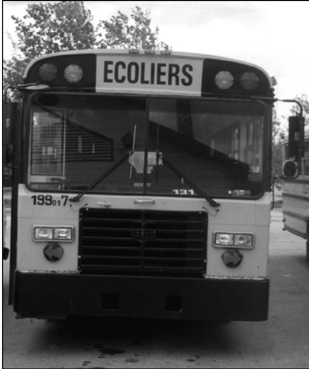
Figure 1 Eight-light system, front view
