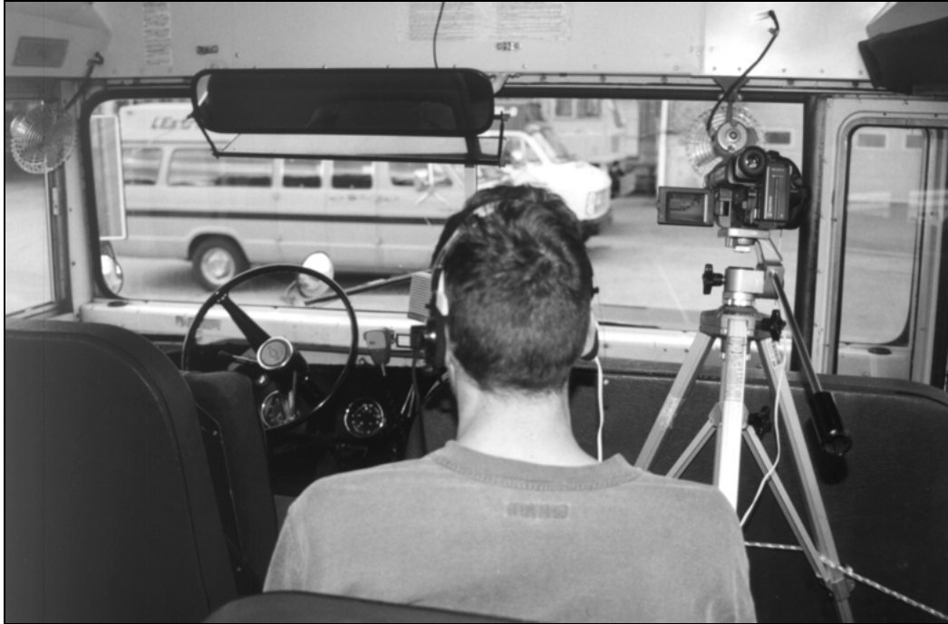
Figure 6 Front camera and observer's position
