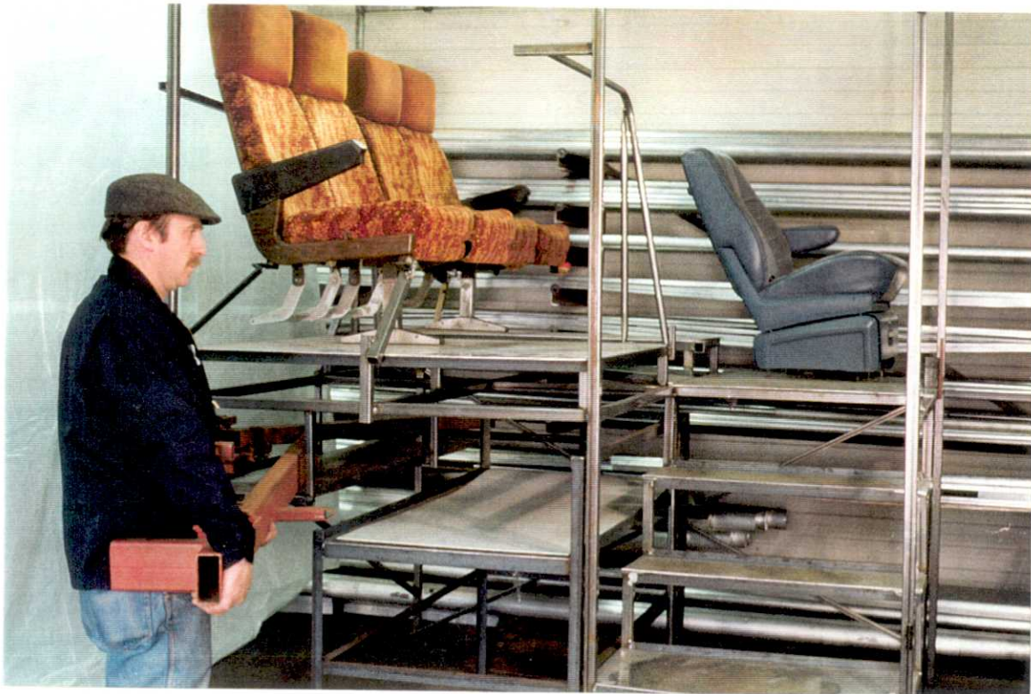
Photo 1: Full size mock-up of front of standard bus showing "twin rails" under seats and folded rail chair behind driver's seat.
