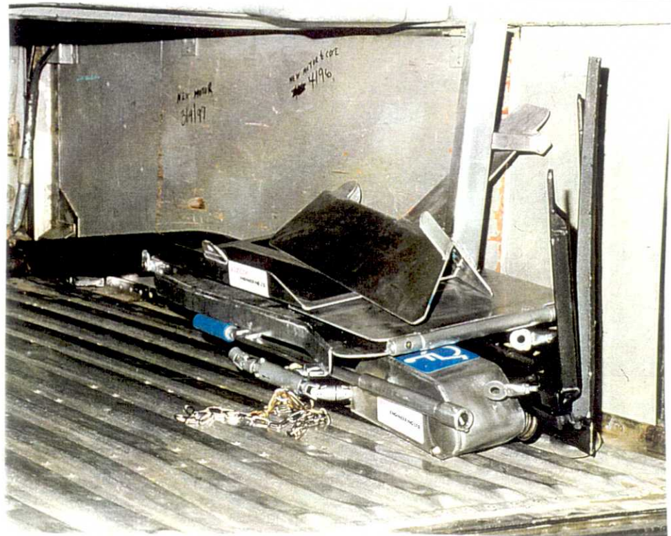
Photo 25: Monorail components in bus baggage tank. Note: these components would be in a custom box in actual service.
