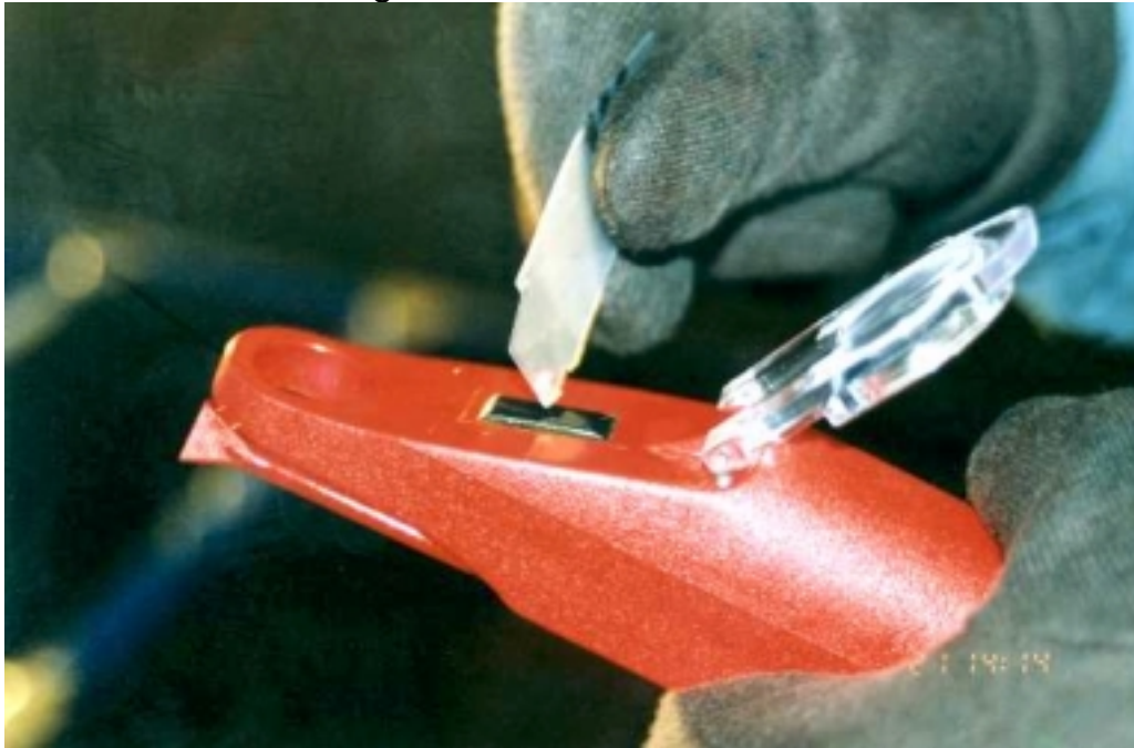
Photo 2.7 Using a Brix-Scale Refractometer
