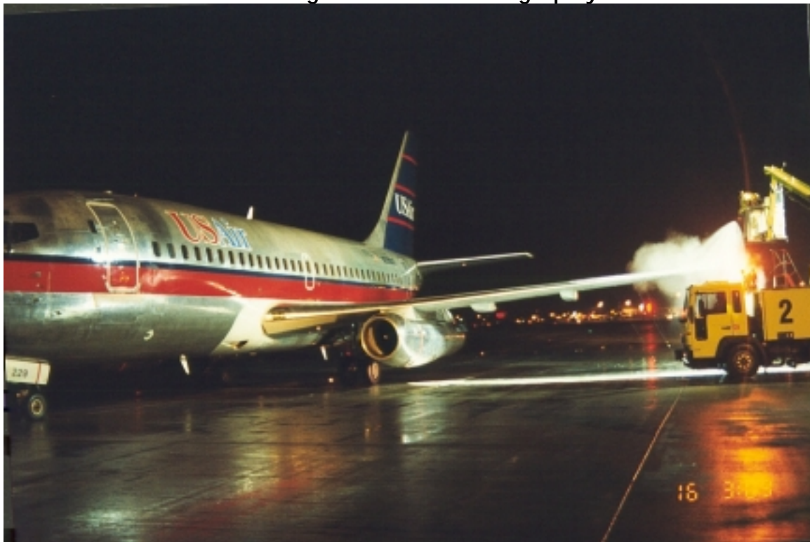
Photo 2.26 Removing Snow with De-icing Spray
