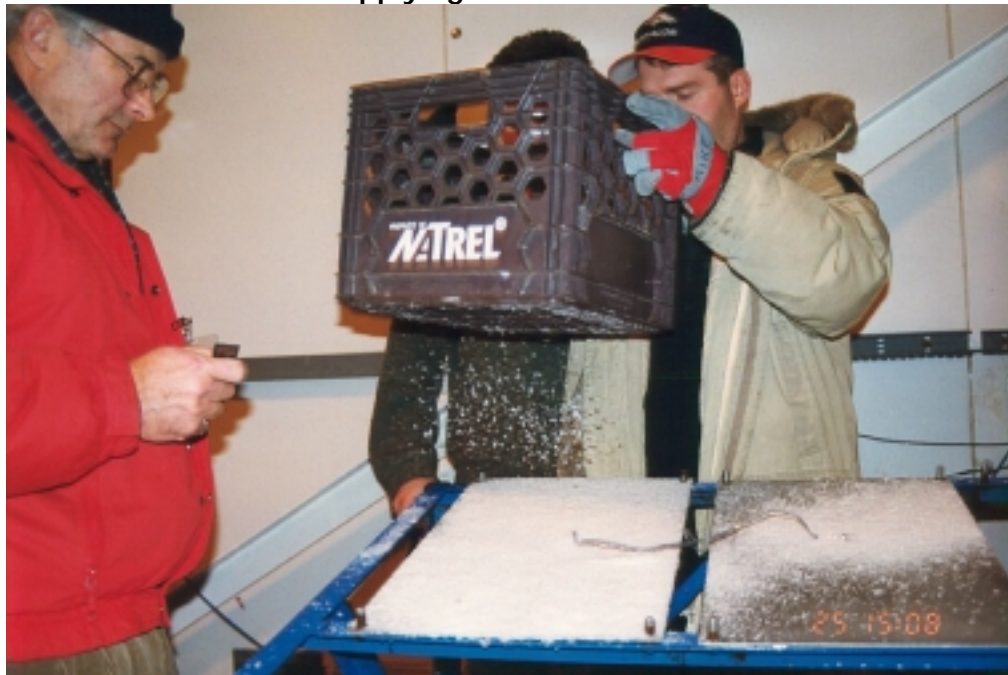
Photo 2.21 Applying Snow to Plate
