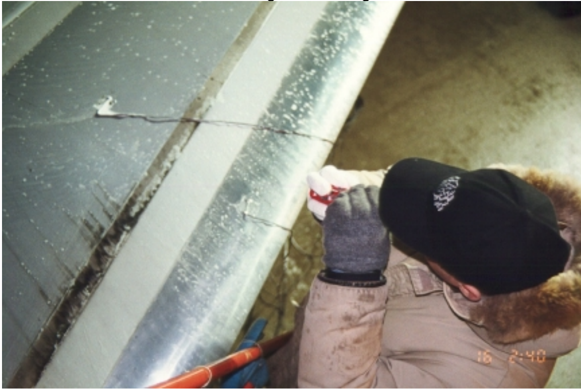
Photo 2.27 Measuring Fluid Strength
