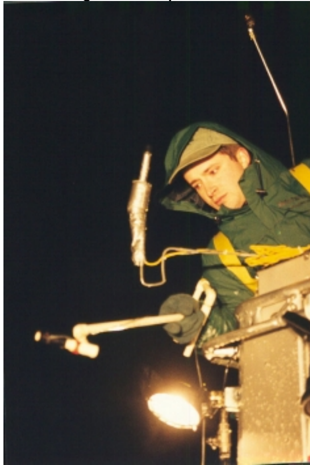
Photo 2.2 Measuring Fluid Temperature at Wing
