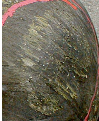
Figure 4: Damage Due to Cylinder Drop.
