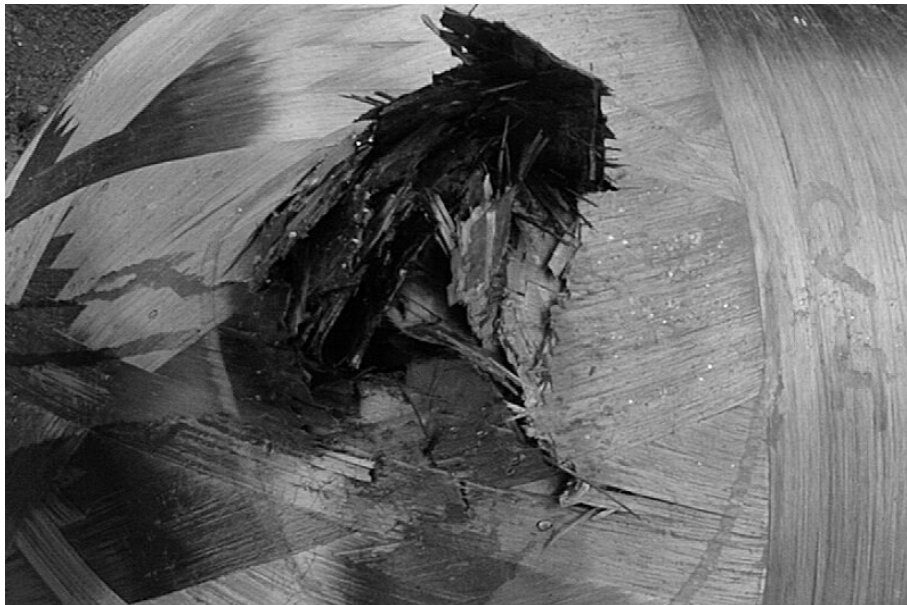
Figure 5: Failure of the Cylinder
