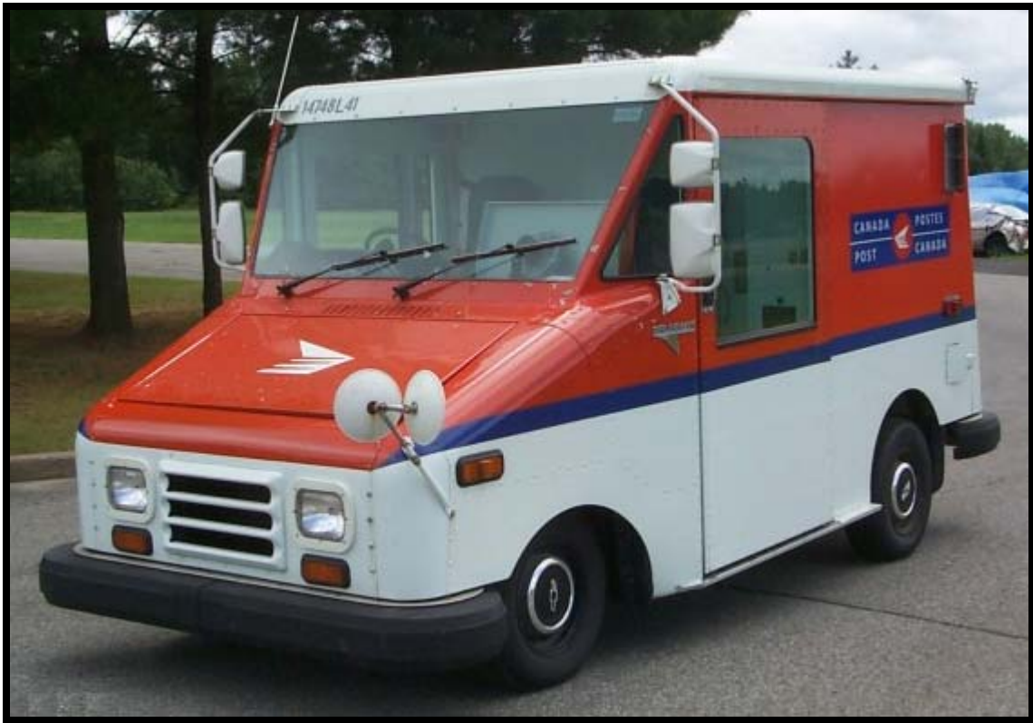
Canada Post Solectria-Grumman LLV Electric Postal Delivery Truck
