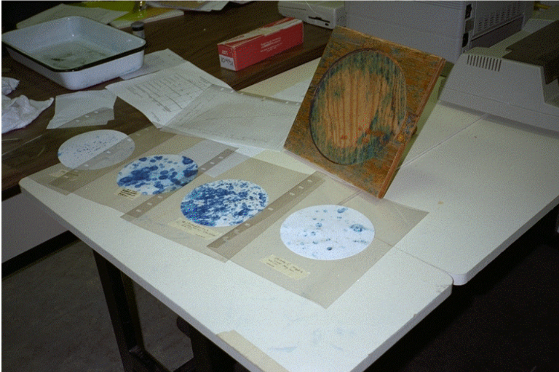
Examples of Droplet Sizes Produced by National Research Council Canada's Spray System
