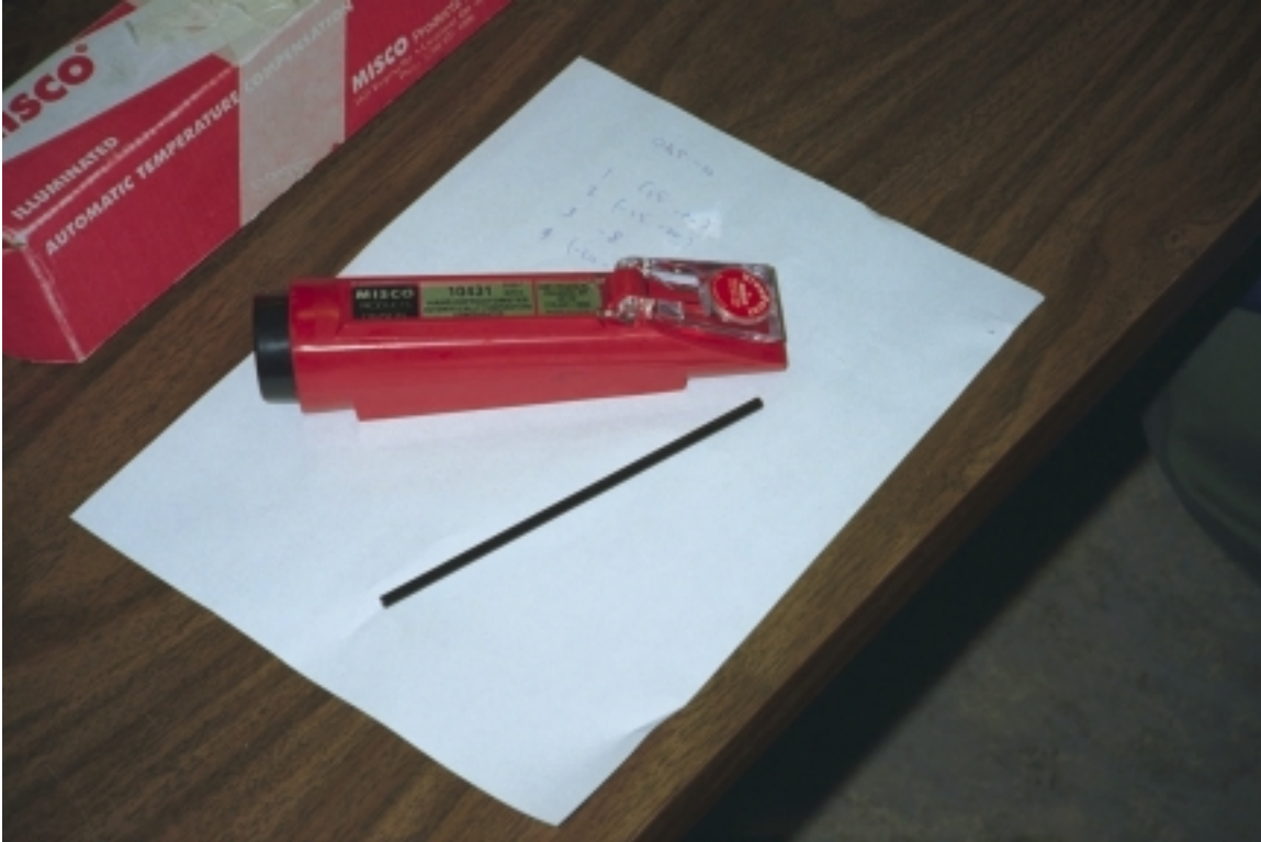
Photo 2.13 Misco Refractometer Used to Measure Freeze Point
