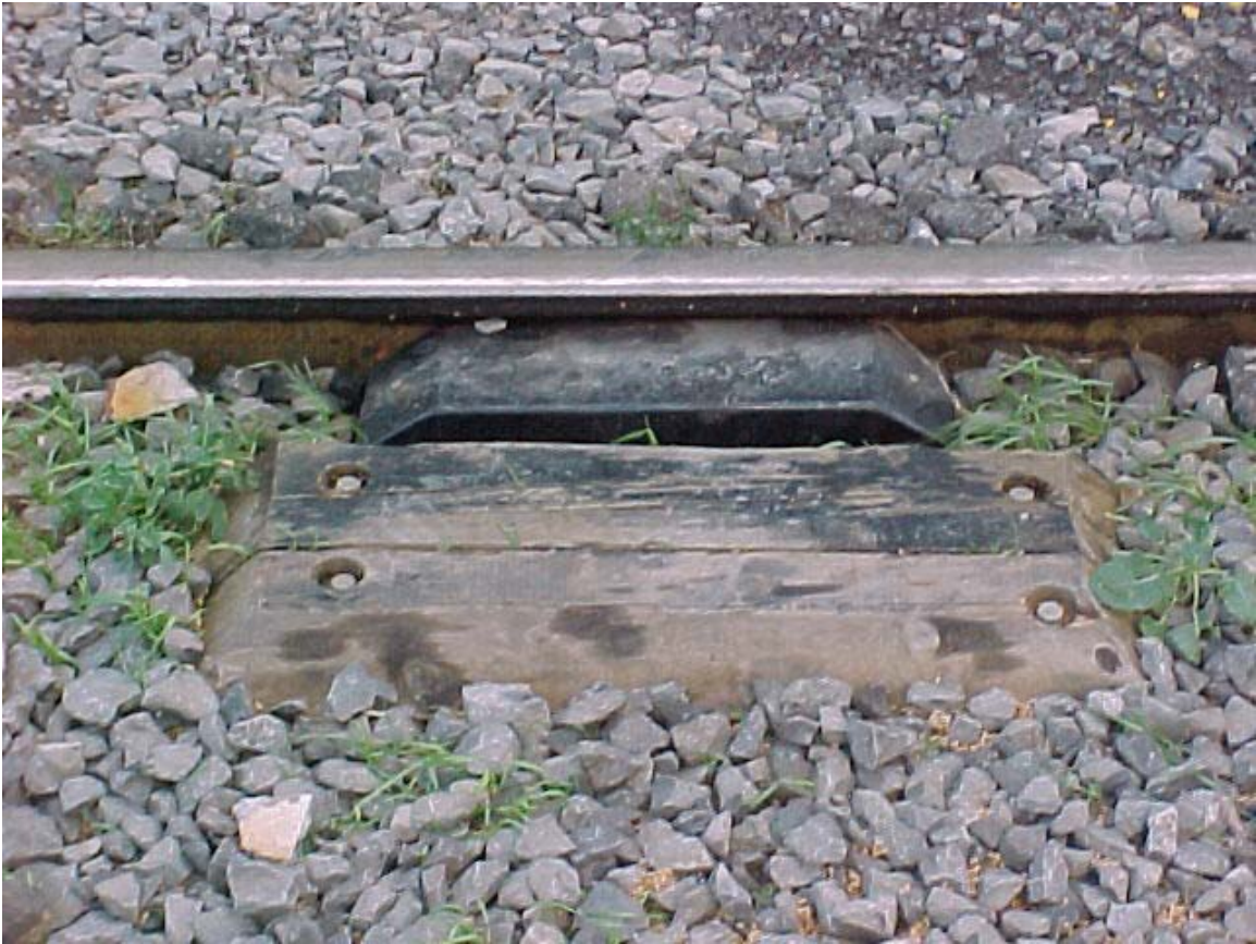
Figure 21 Eastbound wheel sensor
