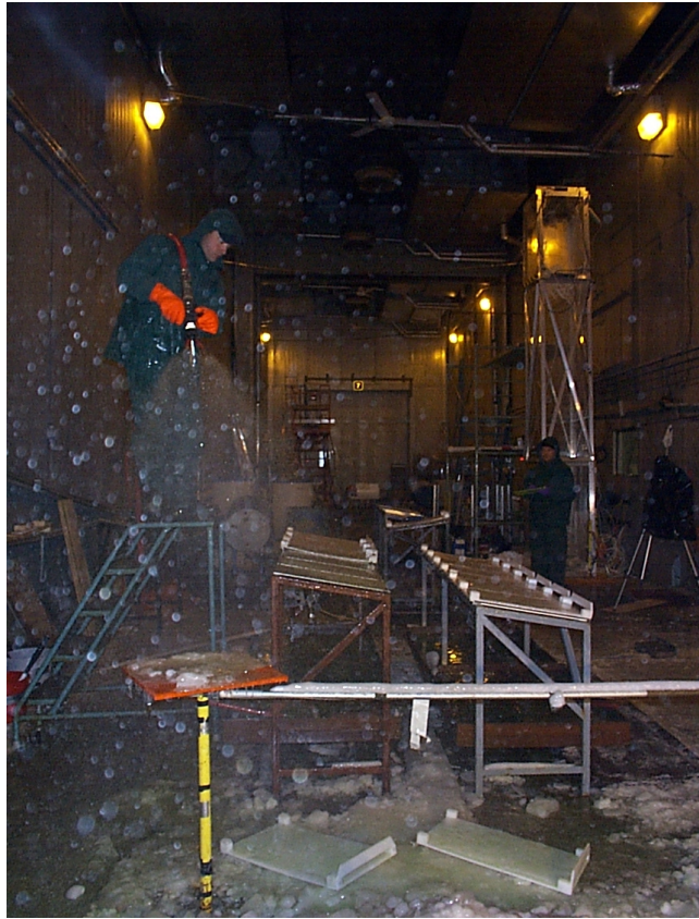
Photo 2.15: Spraying Type IV Fluid
