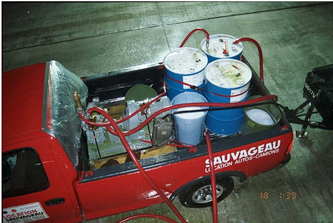
Photo 2.7: Mobile Type IV Fluid Sprayer Unit
