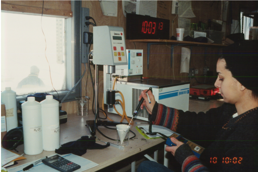
Photo 2.3: Temperature Measurement Before Conducting Viscosity Test
