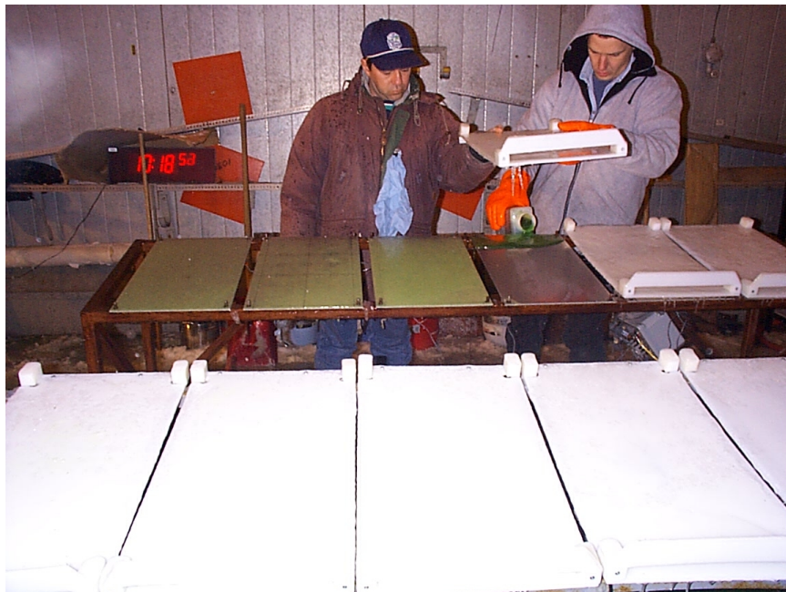
Photo 2.16: Pouring of Type IV Fluid
