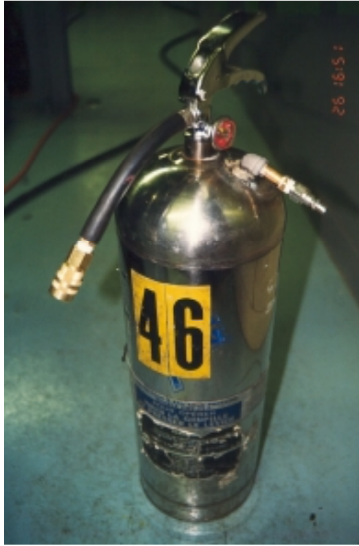
Photo 3.1: Hand-Held Sprayer for Deicing
