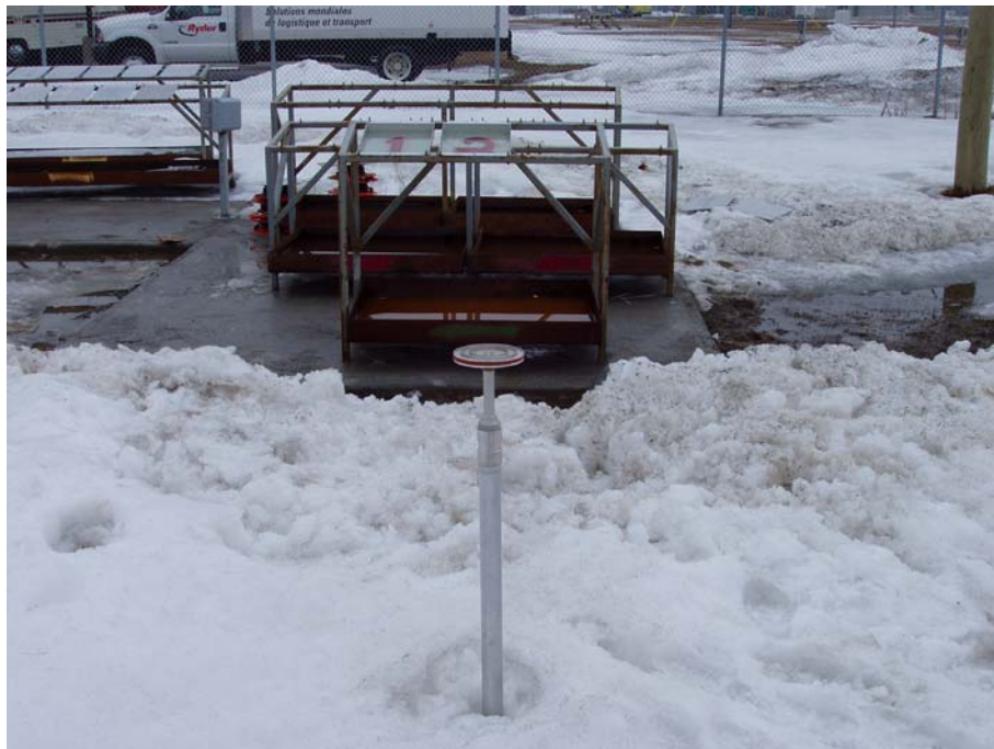
Photo 2.2: Hot Plate Snow Gauge and Test Stand with Precipitation Pans
