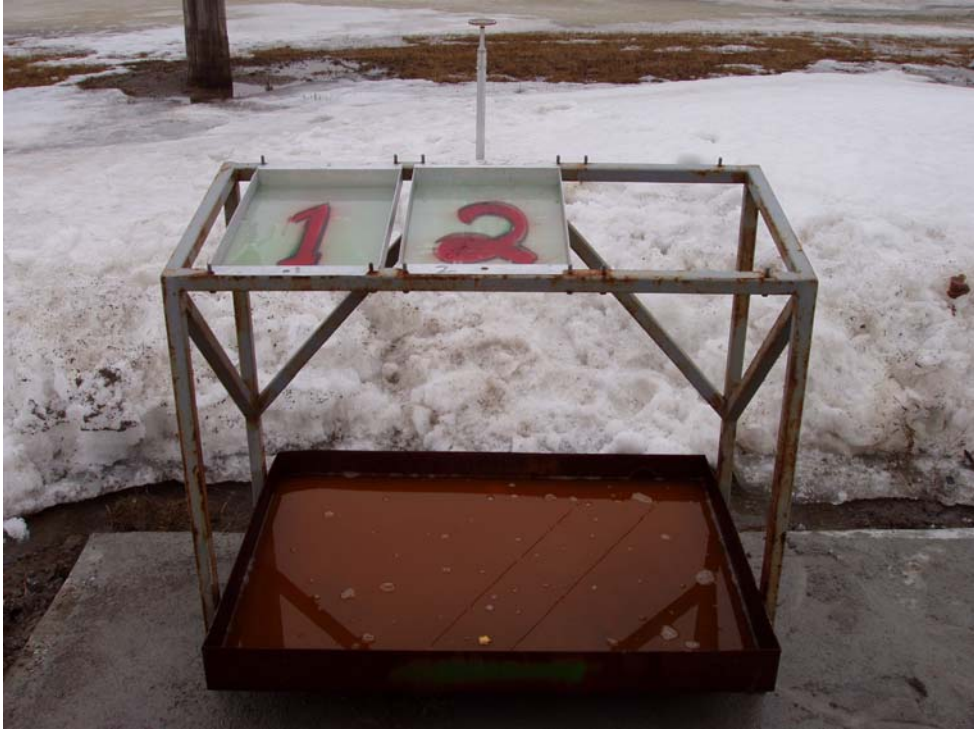
Photo 2.3: Test Stand and Precipitation Pans
