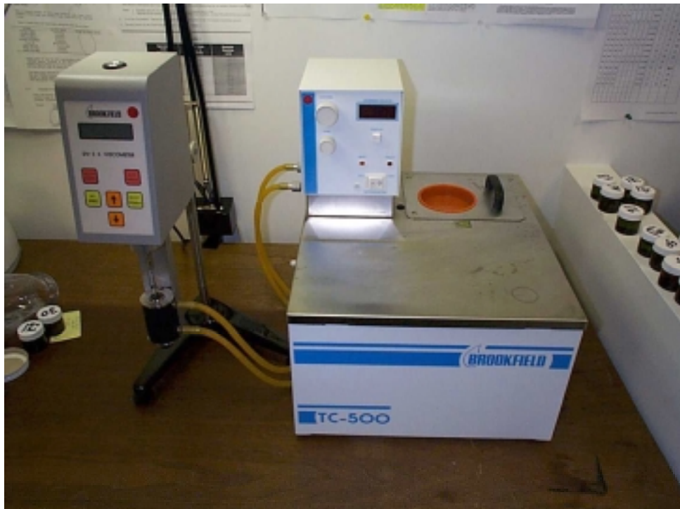
Photo 2.12: Brookfield Digital Viscometer Model DV-1+ and Temperature Bath
