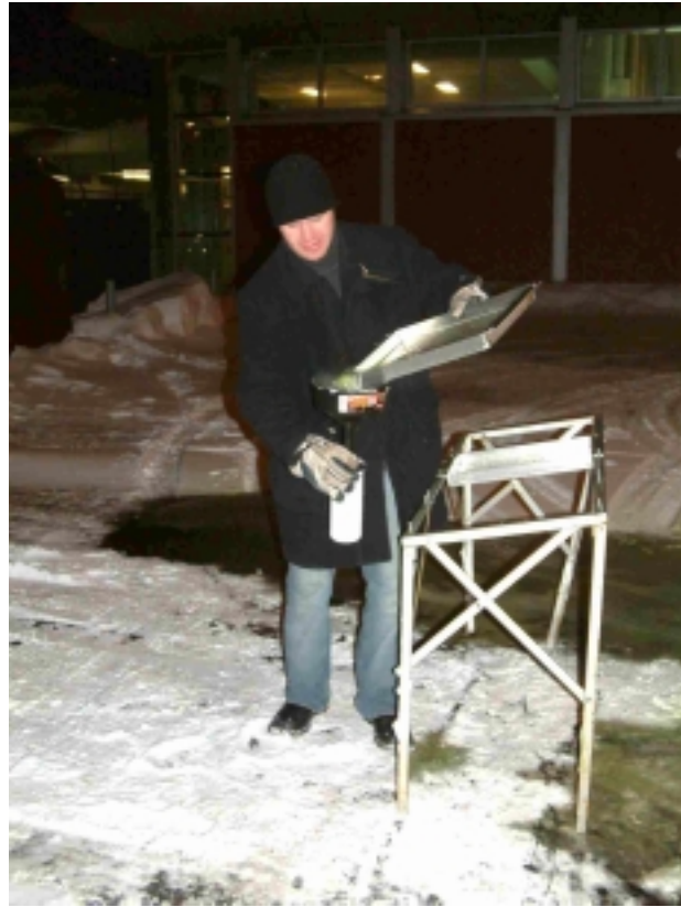
Photo 2.7: Transferring Type IV Fluid from Rate Pan to 1 Litre Sample Containers
