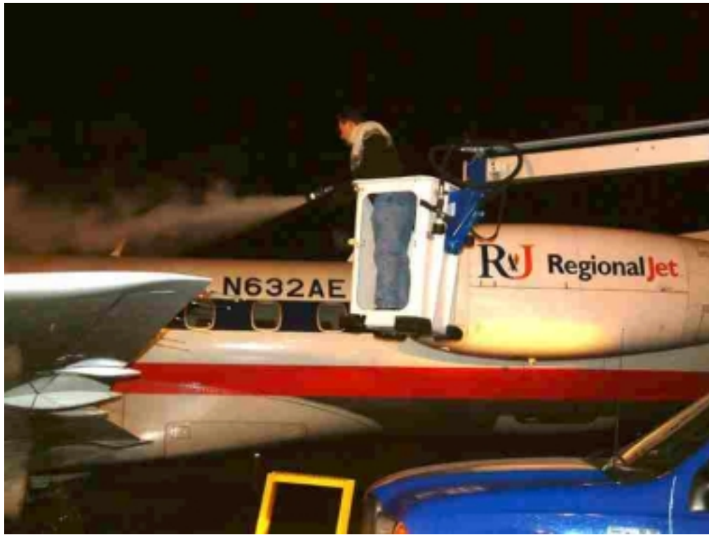
Photo 2.5: Heated Type IV Sprayed onto the Wings of an EMB-145 in DBQ
