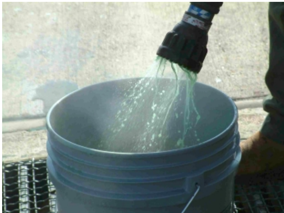
Photo 2.8: Heated Type IV Spray into 20 Litre Containers at DFW
