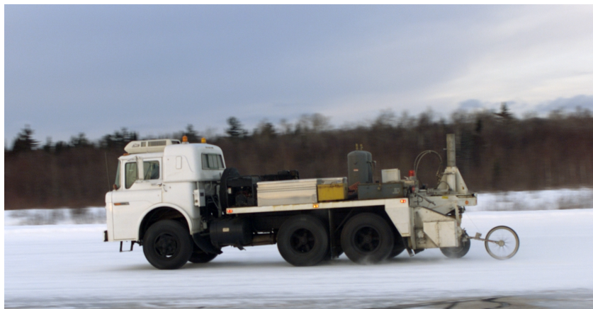
Figure 14. Compacted snow strip on the centre-line of runway 13-31 (a) and the NASA-ITTV on the compacted snow (b) during the afternoon of 05 February 2002
