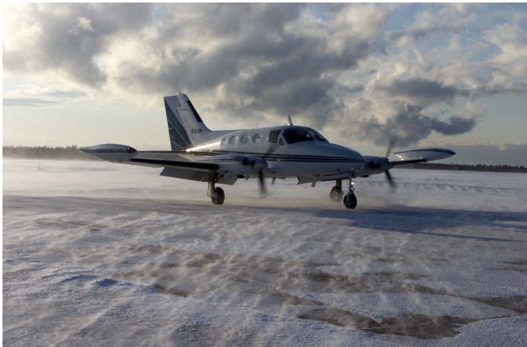
Figure 16. Conditions of runway 13-31 south at 16:25 on 07 February 2002 just prior to aircraft testing, showing (a) blowing snow, almost parallel to the length of the runway and (b) Cessna 414 preparing to test
