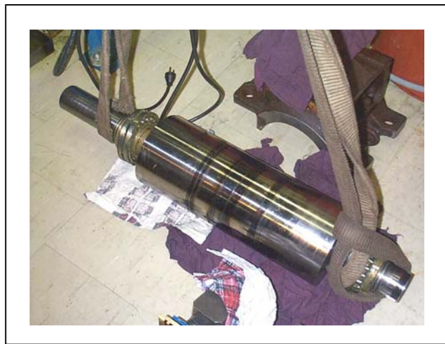
Figure 20 Shaft after failure of the Mark 1 Vespel ® -lined bearing
