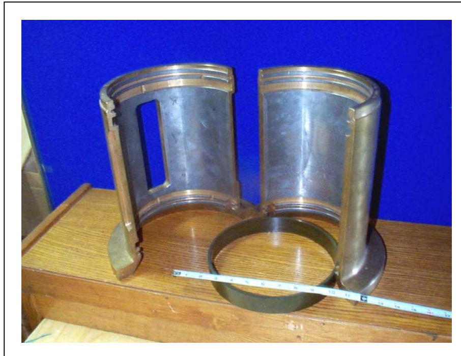
Figure 8 Babbitt-lined traction motor bearing (with Vespel ® ring in the foreground)
