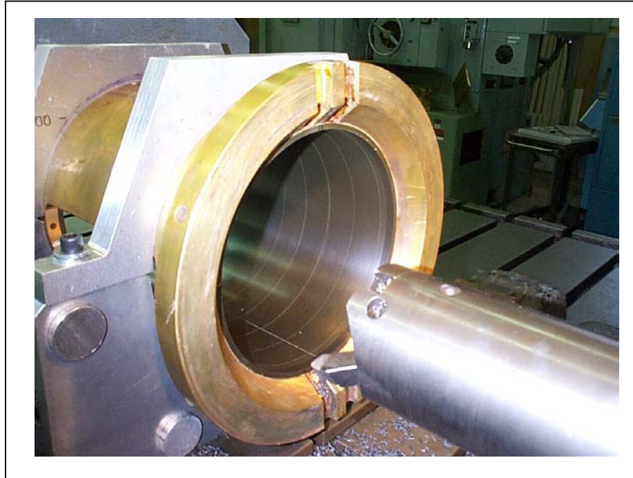
Figure 17 Machining Vespel®-lined bearing
