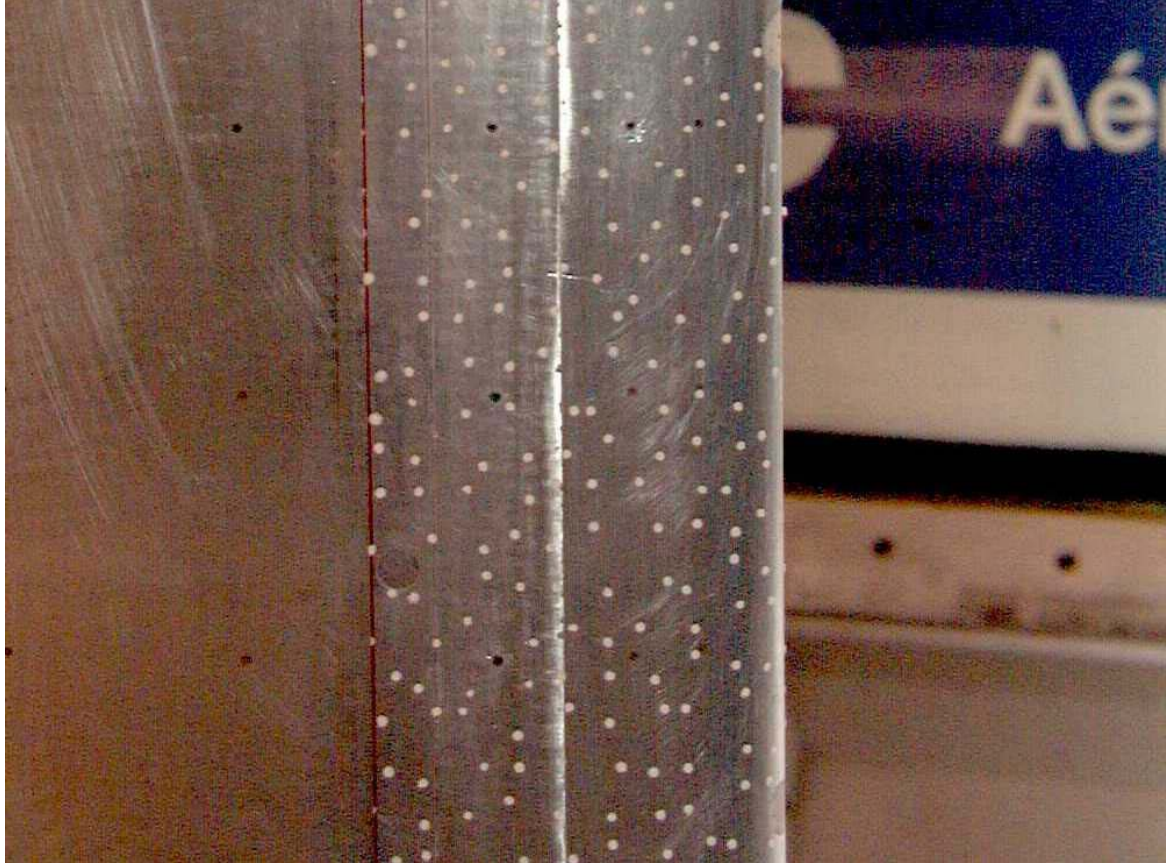
Figure 2 Roughness; k/c = 0.0006 to 0.15c ; \lambda = 140
