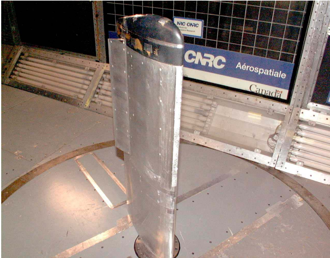
Figure 1b Wind tunnel model with roughness to 0.02c ; \delta = -20^\circ
