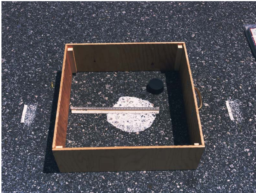
Figure H.8 PSU Volumetric Texture Depth, Glass beads – USA
