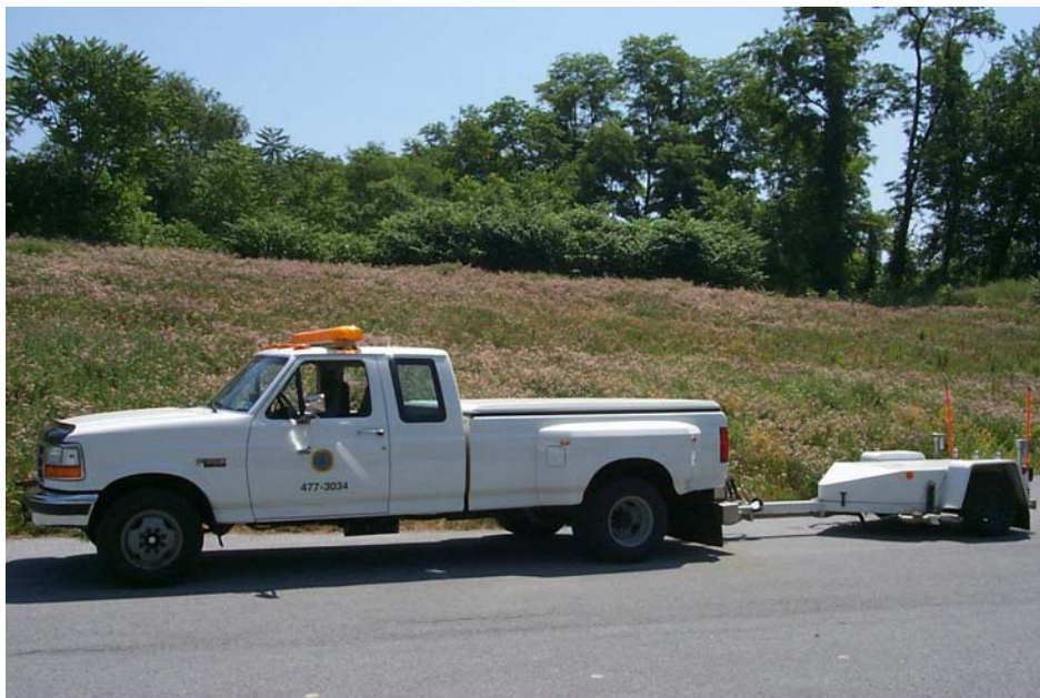
Figure I.22 Pennsylvania DOT E-274 Locked Wheel Tester – USA
