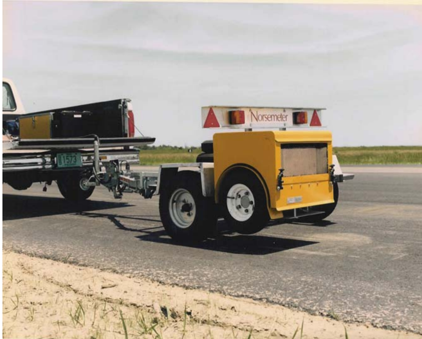
Figure I.17 Norsemeter ROAR (variable slip tester)-Norway
