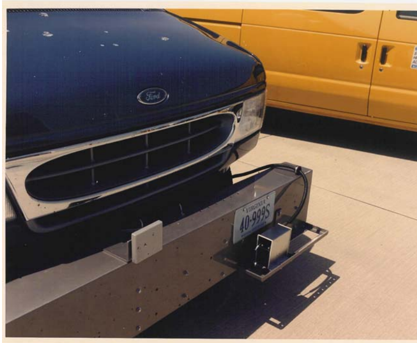
Figure J.11 VA DOT ICC High Speed Profiler-USA
