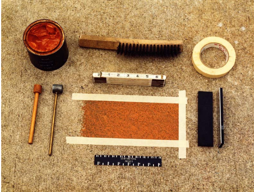
Figure H.7 NASA Volumetric Texture Depth, Grease – USA
