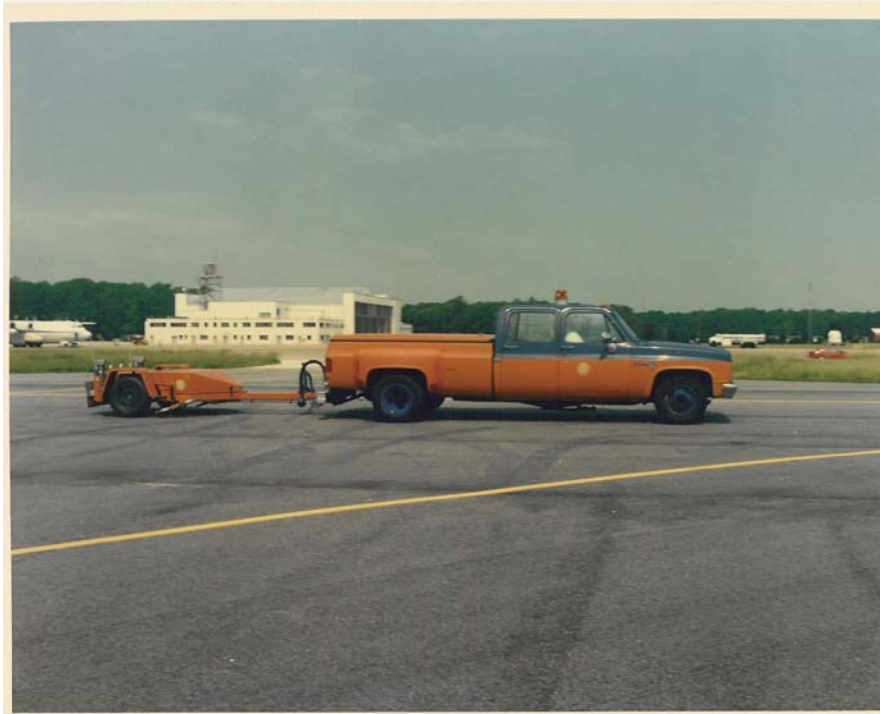
Figure I.15 MD DOT E274 Locked Wheel Tester (SNR) – USA
