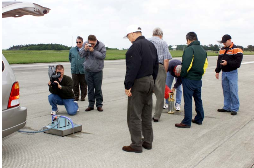
Friction Workshop, NASA Wallops Flight Facility Date: 5/14/02 Time: 14:03:38 Circular Texture Meter and Outflow Meter
