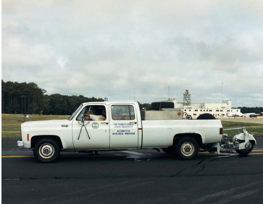
Figure I.21 Penn State E-274 Locked Wheel Tester (SNB and SNR) – USA
