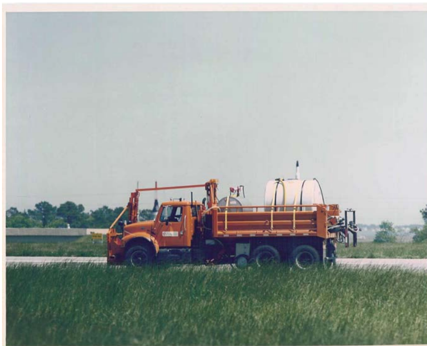
Figure I.19 Norsemeter OSCAR (variable slip tester)-Norway
