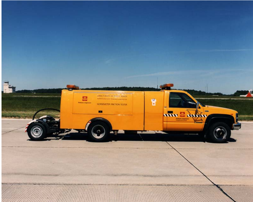
Figure I.19 Norsemeter OSCAR (variable slip tester)-Norway
