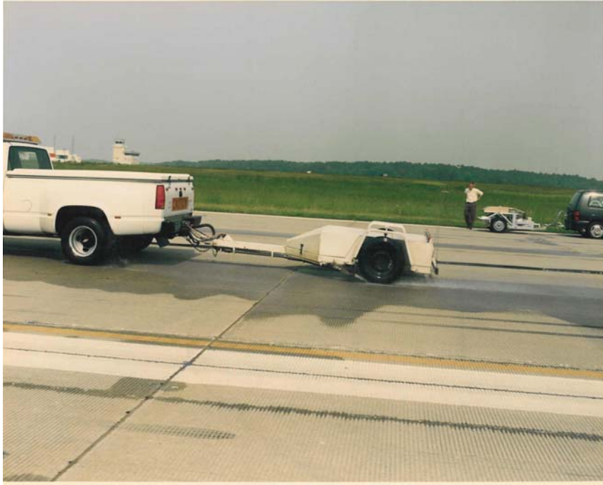
Figure I.13 PTI K. J. Law E-274 Locked Wheel Tester (SNR) – USA
