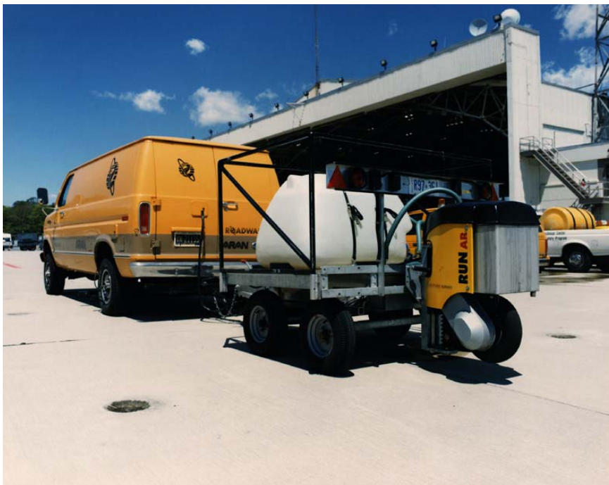
Figure I.17 Norsemeter ROAR (variable slip tester)-Norway
