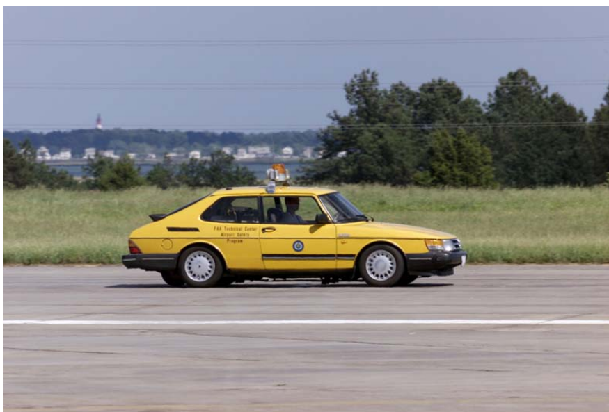
Friction Workshop, NASA Wallops Flight Facility Date: 5/15/02 Time: 15:36:46 FAA SAAB Friction Tester
