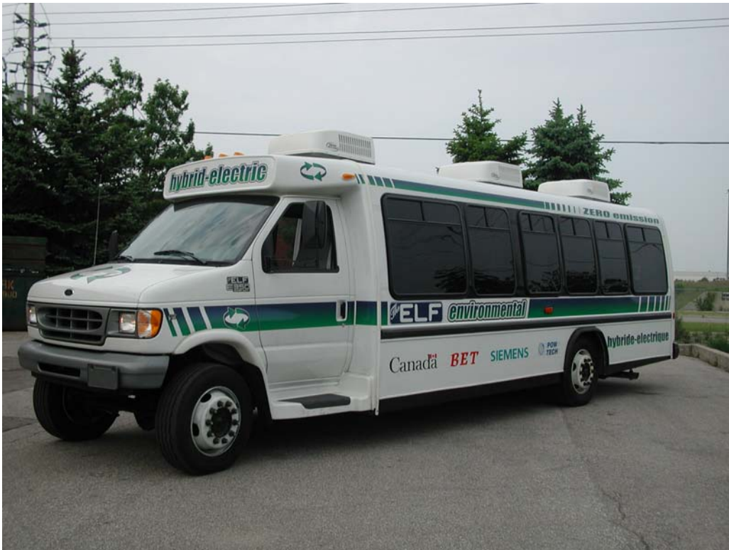
Figure 1 Prototype 28 ft. ELF multi-mode hybrid electric shuttle bus
