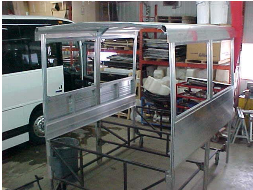
FIGURE 9: Säffle System 2000 Bus Cross-Section Mock Up
