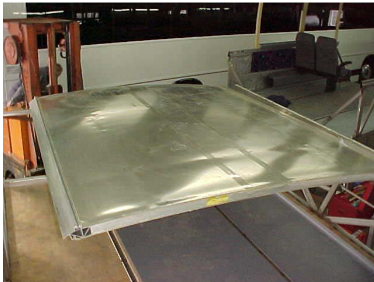
Figure 7.5: Completed Panel for the Roof
