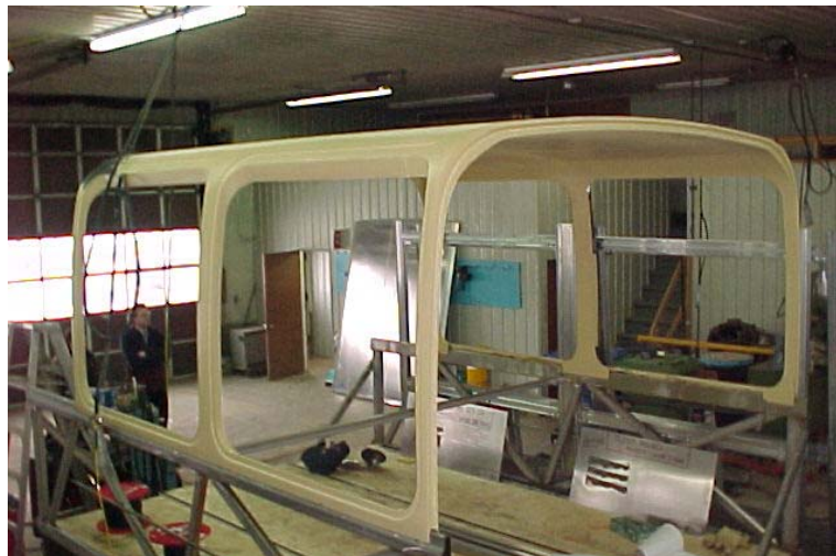
Figure 7.3: Composite Roof Module Prototype
