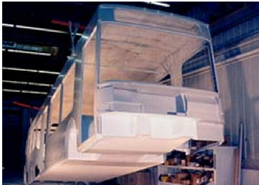
Figure 4.2: NABI CompoBUS One-Piece Composite Structure (Photo courtesy of North American Bus Industries, Inc.)
