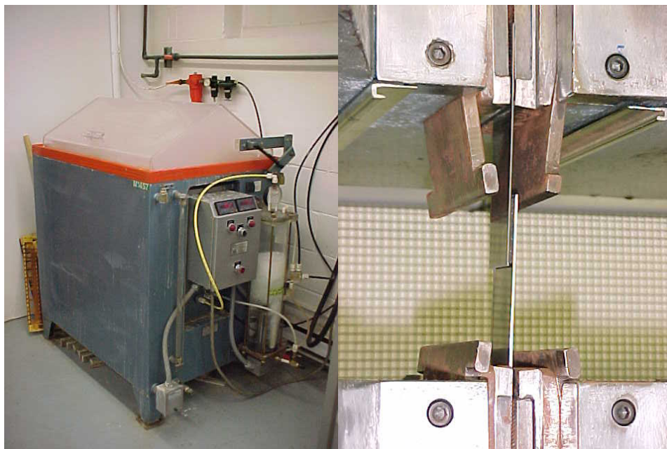
Figure 6.12: Salt Spray Testing Apparatus and Tensile Test
