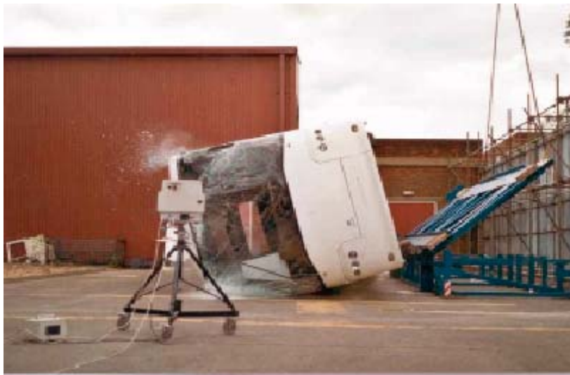
Figure 4.5: R66 Testing of BOVA Magiq Coach at the Cranfield Impact Testing Centre
