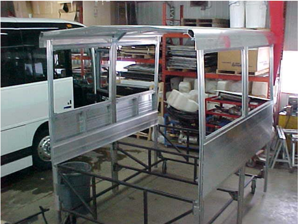
Figure 7.8: Säffle System 2000 Bus Cross-Section Mock Up
