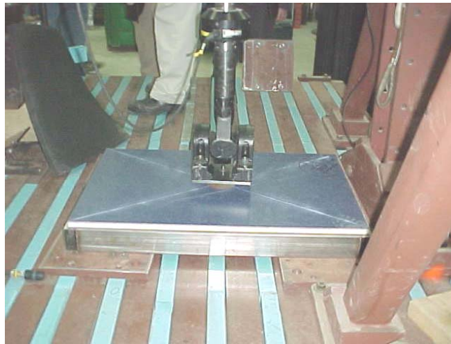
Figure 6.5: New Floor Design Sample Being Tested for Stiffness Properties
