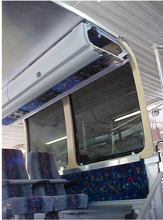
FIGURE 8: Mock-Up Installation of the Sandwich Panel Roof Design
