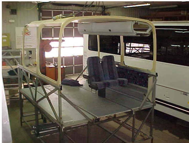
Figure 7.4: Completed Vehicle Cross-Section Prototype, Composite Roof Module and Floor Design 1
