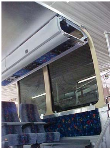
Figure 7.7: Completed Mock-Up Section of the Sandwich Panel Roof Design
