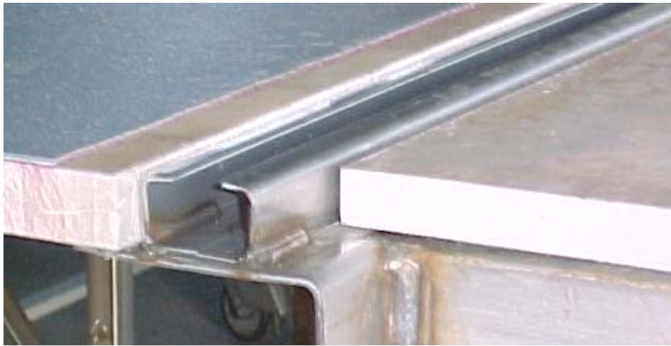
Figure 6.14: Seat Track/Floor Configuration
