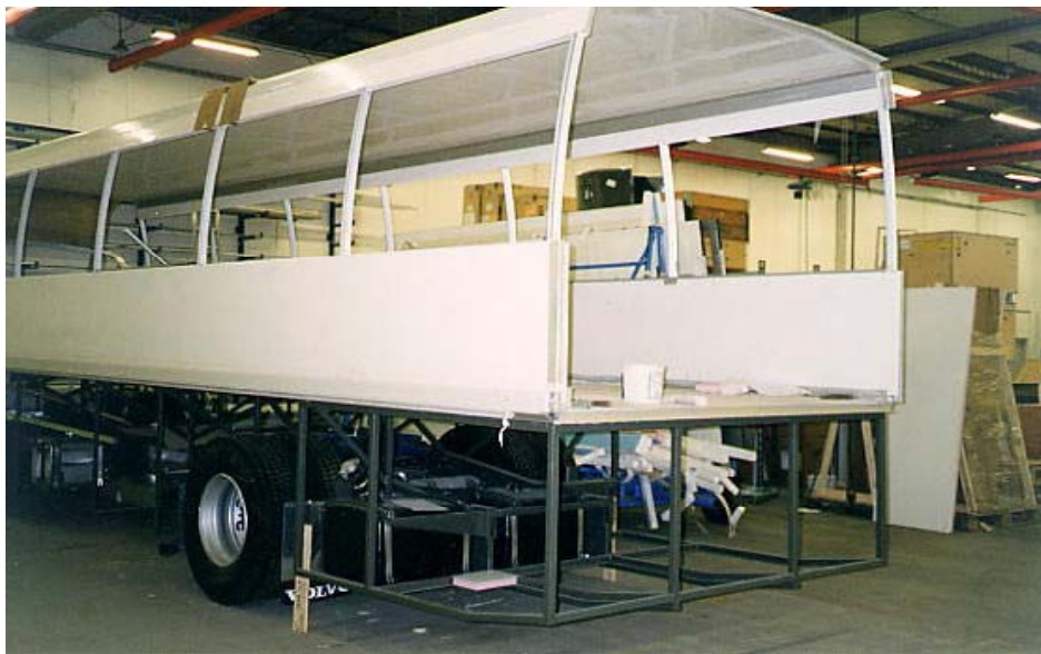
Figure 4.8: Example of D-Bus Body over Chassis Concept (Photo courtesy of Volvo)
