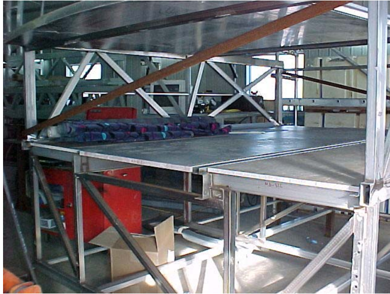
Figure 7.2: New Floor Sample Fitted to XLII Structural Mock Up
