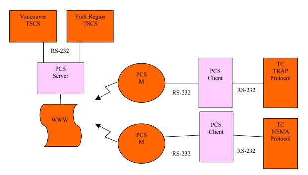
Multiple Protocols and Controllers using 1xRTT Communications
