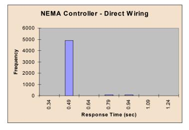
The base line response time measurements for the TRAP and the NEMA protocols summarized in the two histogram graphs. The above graphs clearly indicate the response times for the traffic controllers are deterministically contained within 1 second. However, the bulk of the responses are much less than ½ second.
