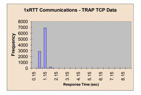
The communications over the 1xRTT did not differ between the bench tests and the field tests as expected. The average response time of the UTCS application over the 1xRTT network was measured to be less than 0.75 seconds for the total set of 27,000 packets of sample data.
