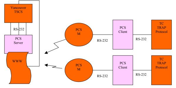
Each TC receives a unique IP address from the service provider and these IP addresses are mapped to the controllers configuration in the system database.
