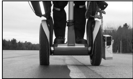
Close-up of Segway showing deflated right tire (on left)
