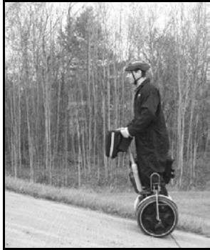
Side view of rider and Segway climbing a 30° hill
