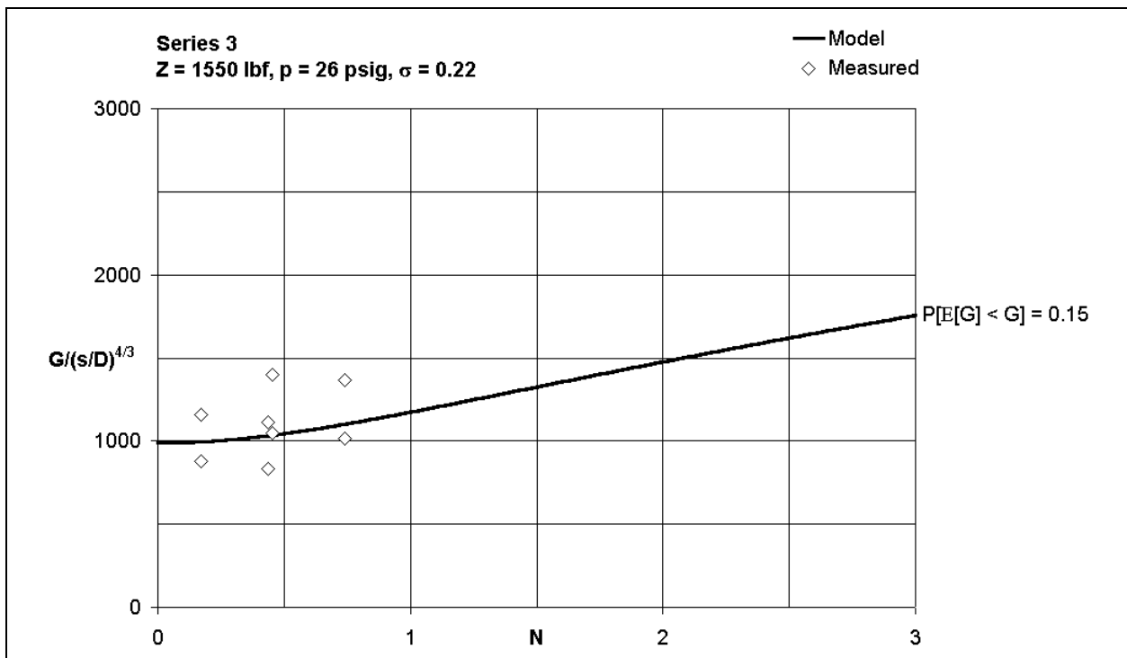
Figure 5.27: Effect of speed number on decelerating force parameter – CRREL vehicle (Series 3)
