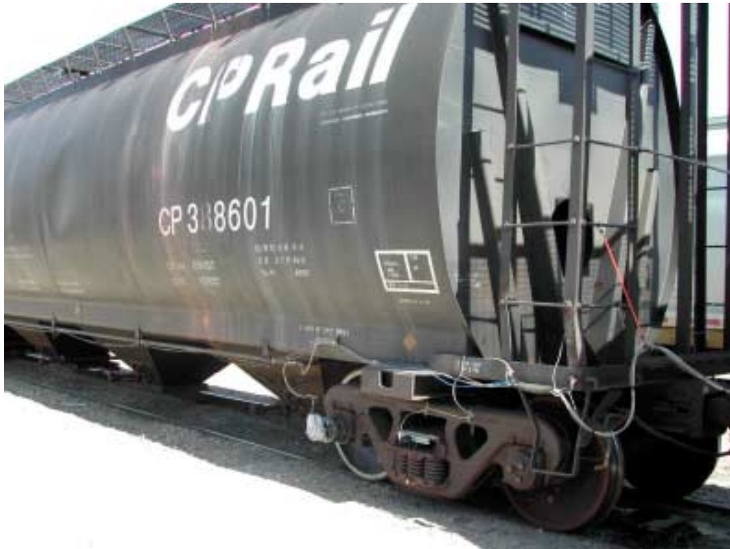
Figure 3 Trailing end of loaded hopper car with instrumentation installed
